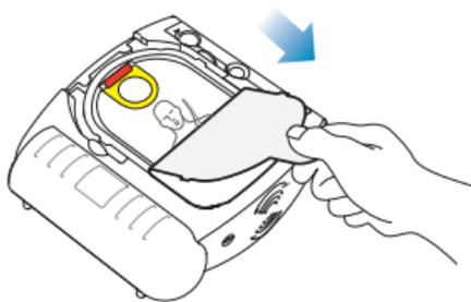
Inside are two pads on a yellow plastic liner. Lift the pads out of the cartridge. You will notice a picture on each pad showing where to place it on the patient.
