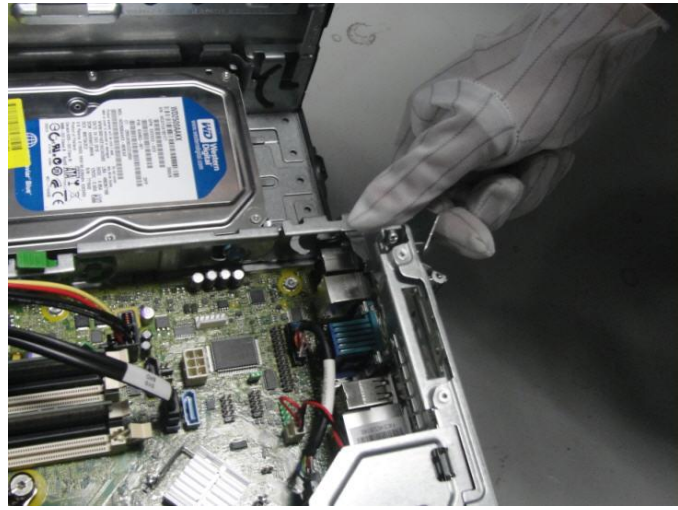
Figure 12 Loose PCI latch cover from chassis
