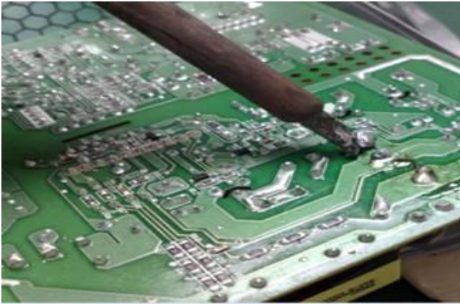
Figure 45 Heat the solder of Electrolytic Capacitors greater than 2.5cm in diameter or height
