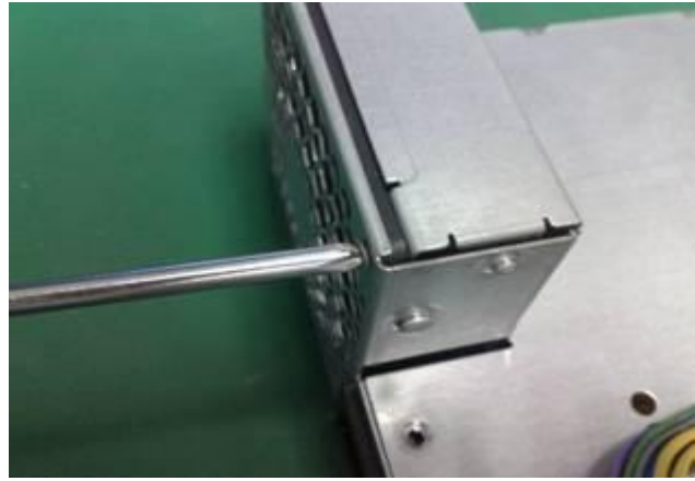
Figure 40 Remove the four screws on the board
