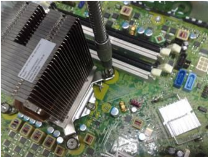
Figure 31 Loose the screws and remove heat sink
