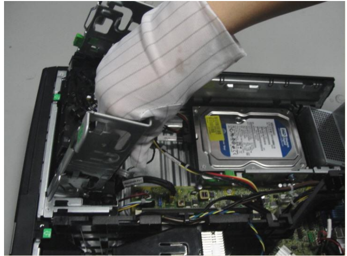
Figure 4 Remove fan duct from the board
