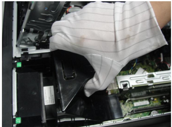
Figure 4 Remove fan duct from the board
