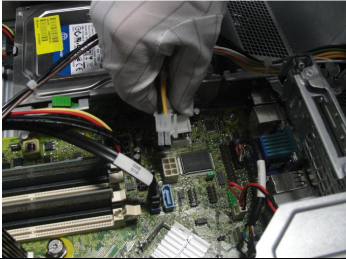
Figure 11 Remove PSU from MB
