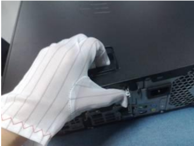
Figure 3 Disconnect the cables from fan duct
