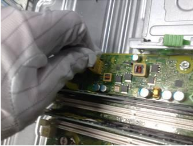
Figure 27 Disconnect FIO cables from MB
