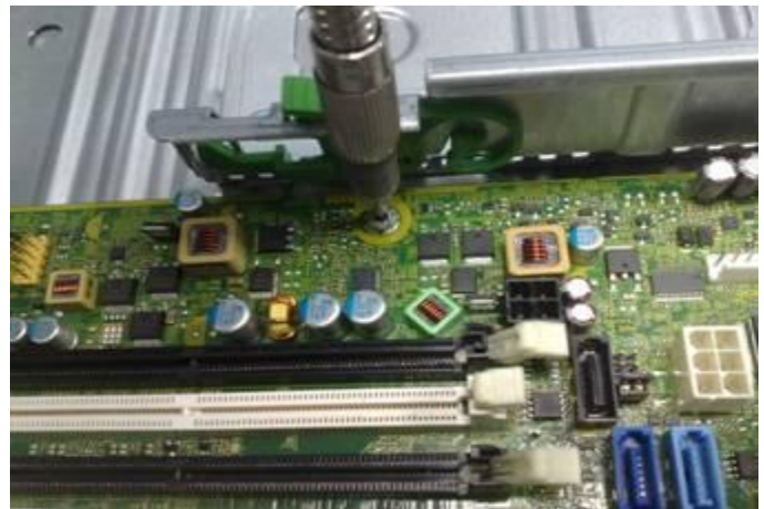
Figure 36 Loose MB screws from chassis
