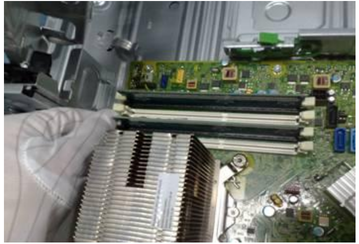
Figure 32 Rotate CPU socket handle and open it up
