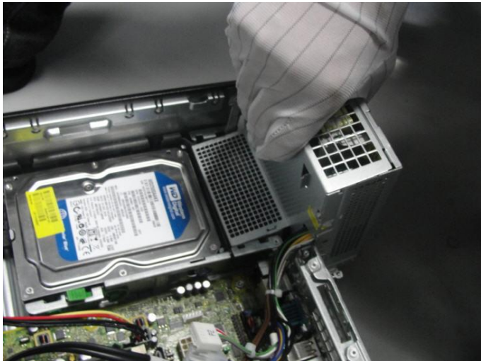
Figure 11 Remove PSU from MB
