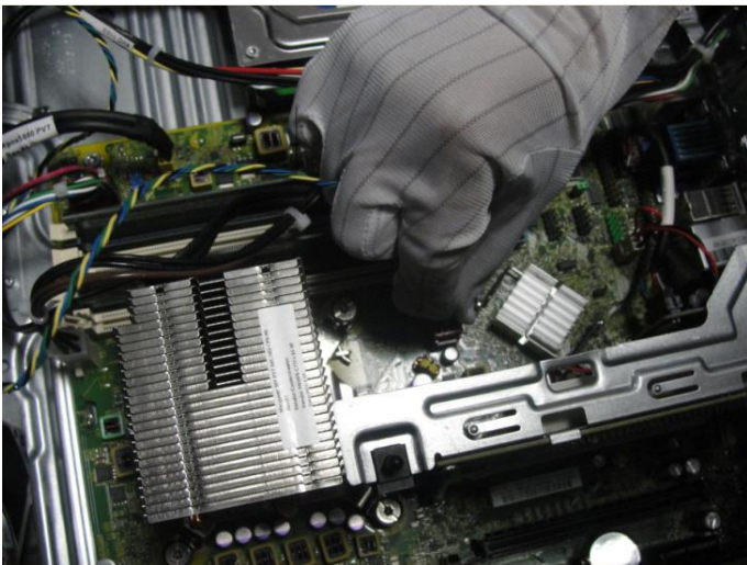
Figure 7 Disconnect front PSU fan cable from MB
