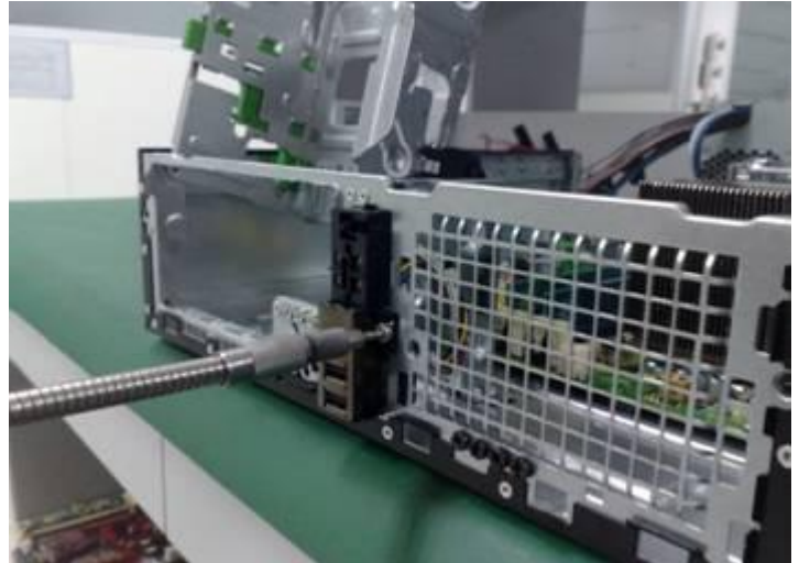
Figure 28 Loose screw of FIO and remove FIO
