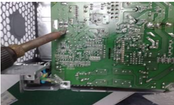
Figure 41 Using Soldering Iron, heat the solder of the cables which connect to the PCA, then remove them
