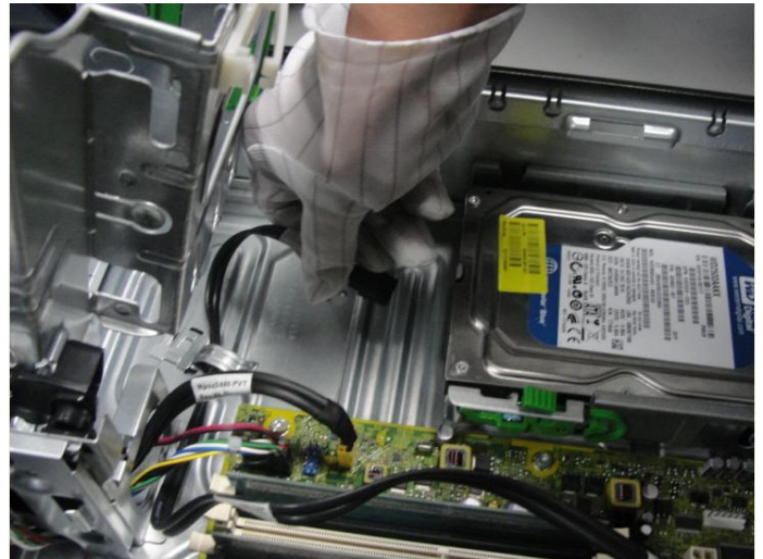
Figure 20 Remove SATA data cable from HDD
