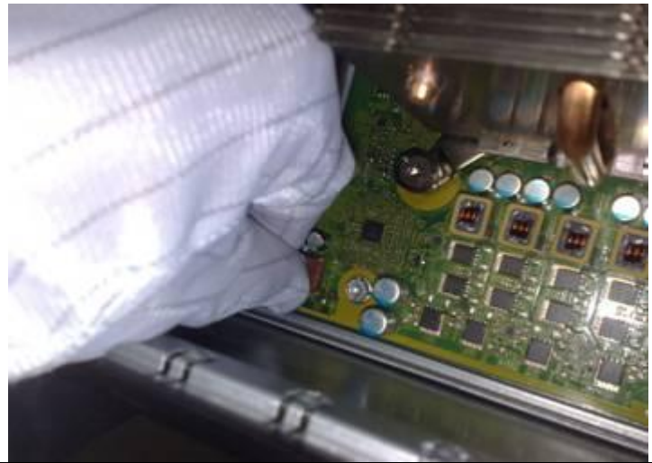
Figure 24 Disconnect front system fan cable from MB
