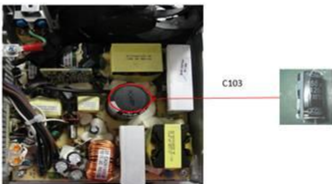
Figure 47 Remove the Electrolytic Capacitors (For Liteon EPA PSU)
