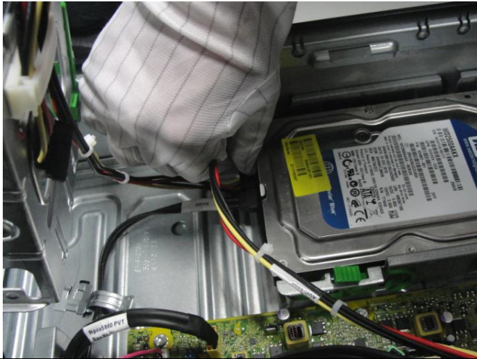
Figure 19 Remove SATA data cable from MB
