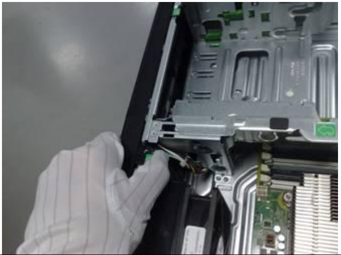
Figure 23 Remove front panel
