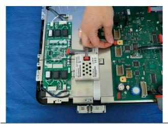
22 Remove the two screws from the IIT module:
