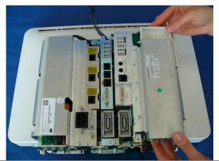
13 Pull back the latch holding the battery and remove the battery:
