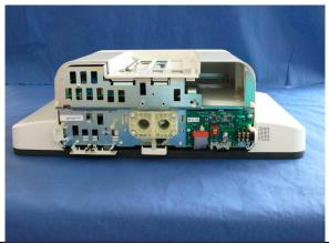
2 Unplug the flat ribbon cable from the Power Switch/ECG Sync Out Board:
