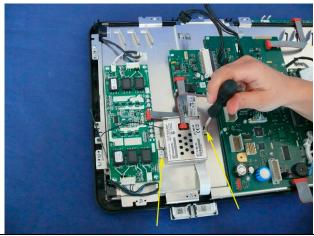
23 Remove the IIT module by pulling it towards you as shown below:
