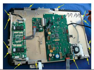
25 Remove the display chassis assembly by pulling it up out of the touch bezel assembly:
