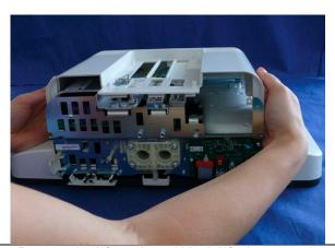
5 Remove the I/O cards and blank I/O slot covers by pushing the release lever and pulling them out at the same time:
