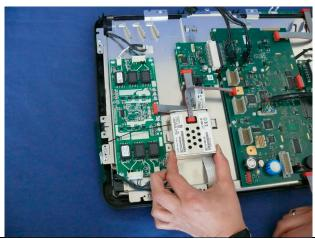
24 Remove the fourteen self-cutting screws from the touch bezel assembly:
