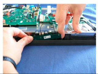
21 Remove the IIT cable from the main board:
