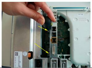
7 Unplug the AC/DC power supply cable by pressing the two latches on the side of the connector:
