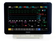
Whether moving a patient throughout the hospital or stationary at the bedside, you won't have to bother with adjusting illumination. The display, with its ambient light sensor, automatically adjusts screen brightness to maintain readability, in nearly any lighting environment.
