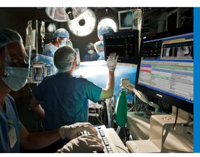
Ambient light adjustment is just part of why the IntelliVue MX550 is an excellent solution for critical care settings and the OR. In the OR, for example, the display automatically adapts to lights being dimmed or brightened during different stages of surgery, reducing overall light pollution in the OR.
