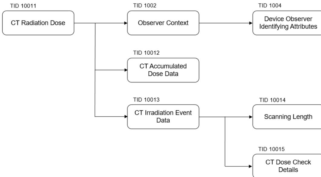
**Figure 20: X-Ray Radiation Dose SR IOD Template Structure**
