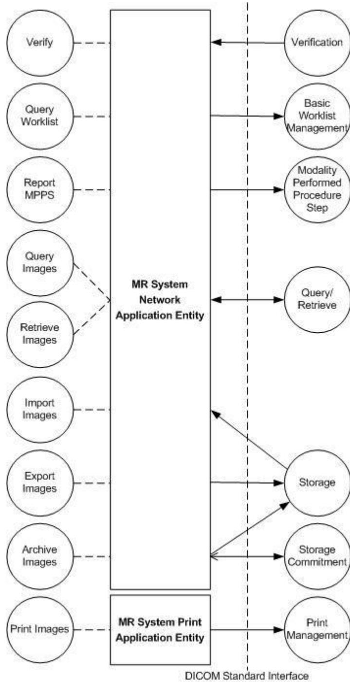
Figure 2: MR System AE Data Flow Diagram
