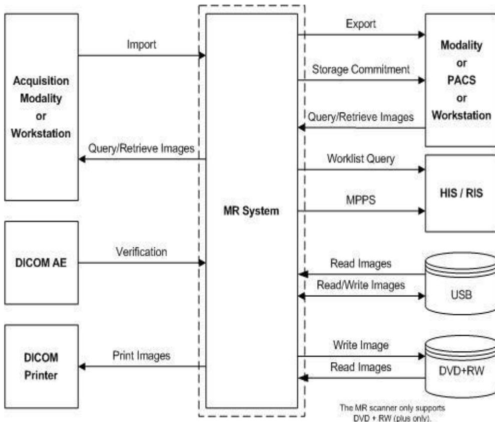
Figure 1: MR System in a DICOM network overview
