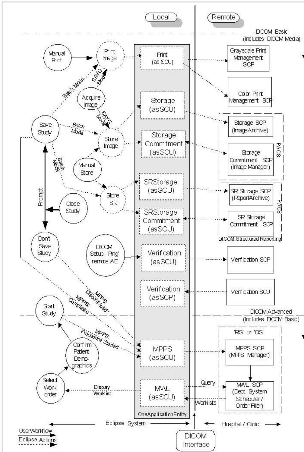
The left side of the diagram (labeled 'Local') represents the HDII system being described in this DICOM Conformance Statement. The right side (labeled 'Remote') represents equipment that HDII is meant to exchange information with (the Hospital/Clinic), and the vertical line in between is the DICOM Interface.
