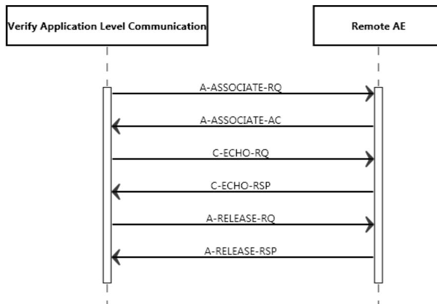
**Figure 4: Sequencing of RWA Verify Application Level Communication**
