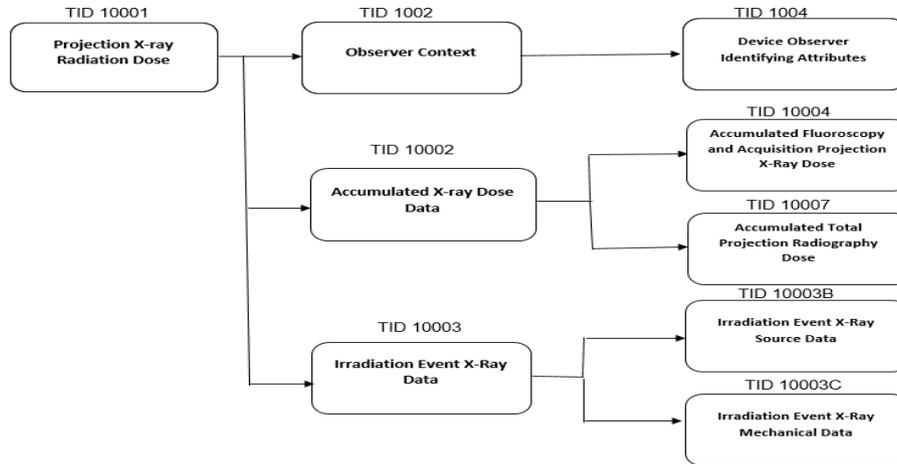
Figure 18: X-Ray Radiation Dose Structured Report IOD Template Structure
