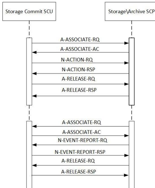
**Figure 9: Data Flow Diagram – Commit Image (asynchronous)**
