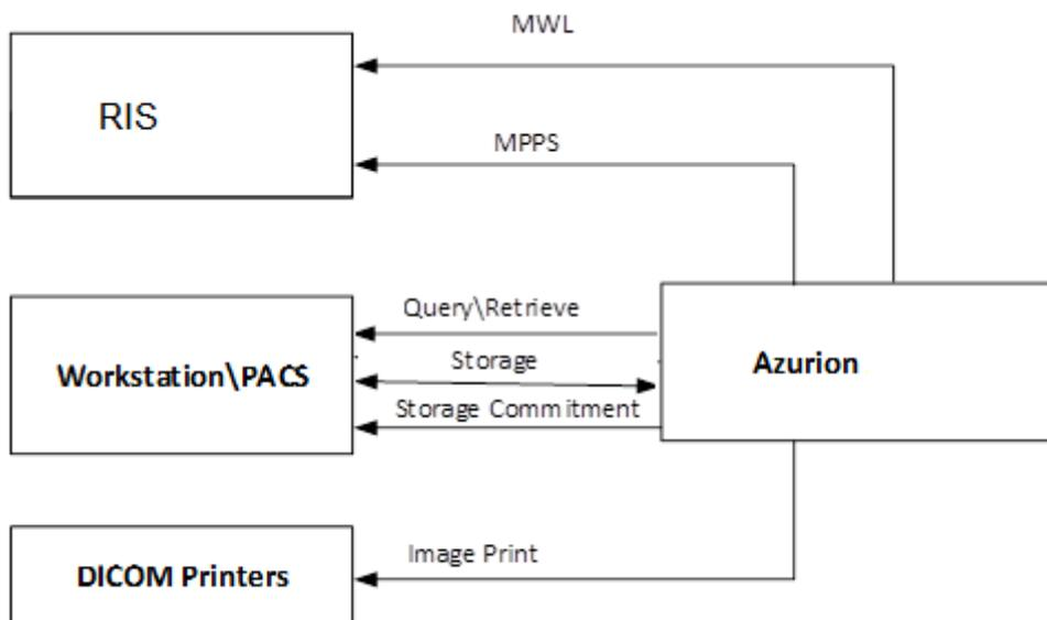
Figure 1 : Data Flow of Azurion R2.1 in a DICOM Network
