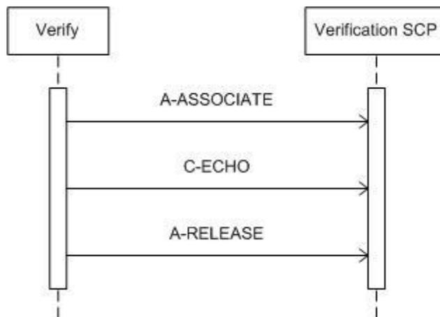
**Figure 6: Data Flow Diagram – Verification as SCU**
