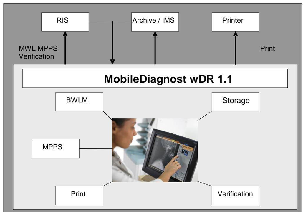
**Figure 1: MobileDiagnost wDR 1.1 in a DICOM network**
