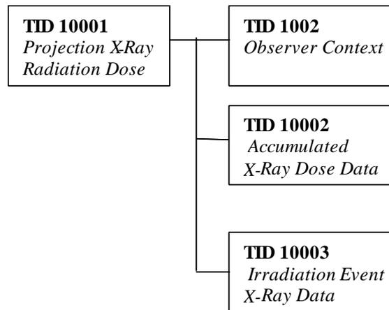
**Figure 14: X-Ray Radiation Dose SR IOD Template Structure**
