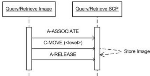
**Figure 6: Data Flow Diagram – MOVE as SCU**
