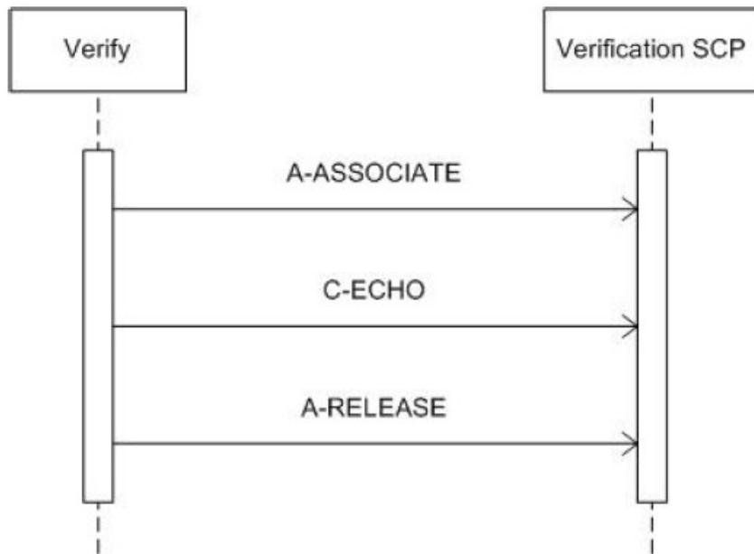
**Figure 4: Data Flow Diagram – Verification as SCU**
