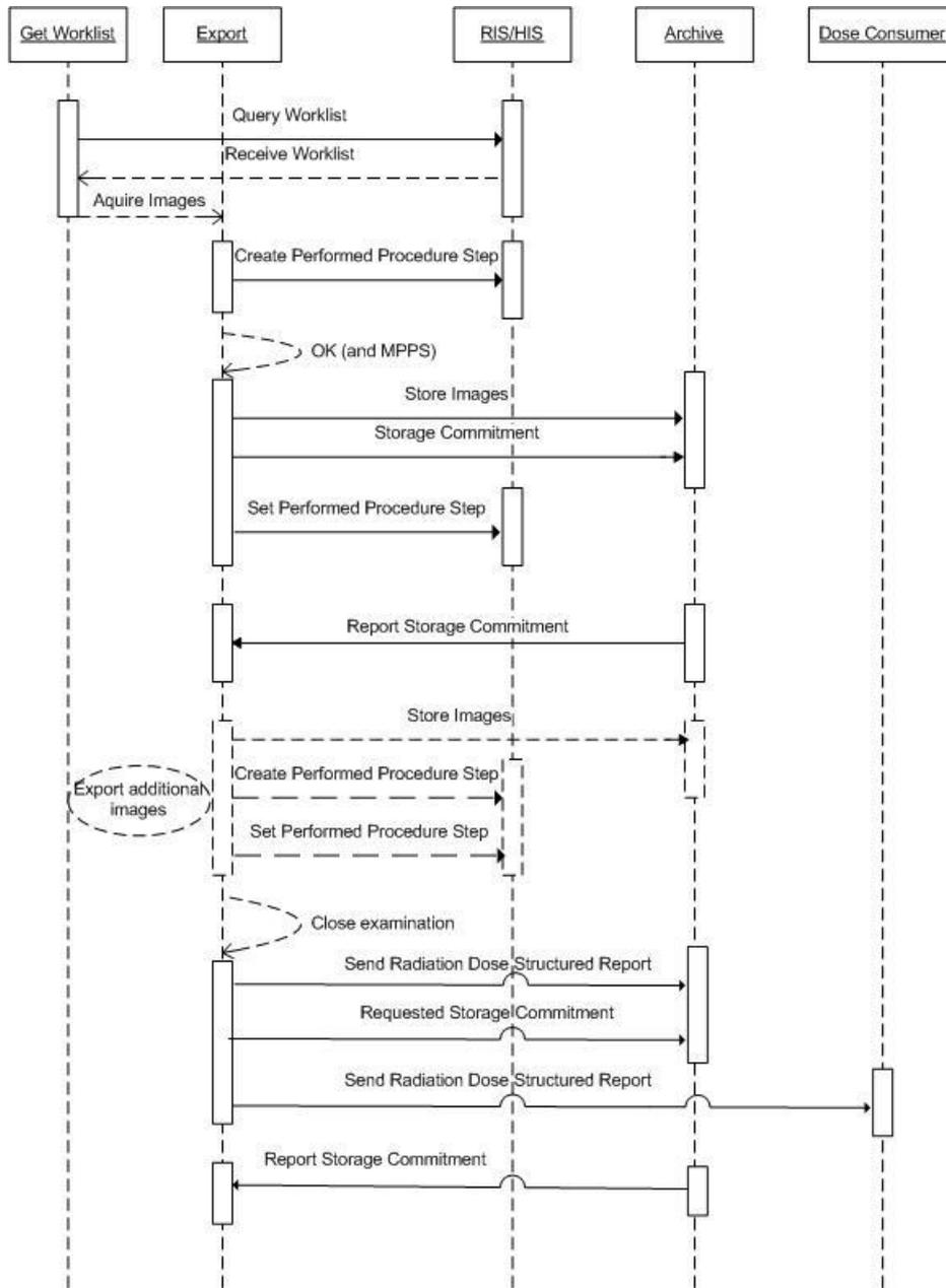
Figure 3: Typical Acquisition Archive Storage Sequencing Constraint.
