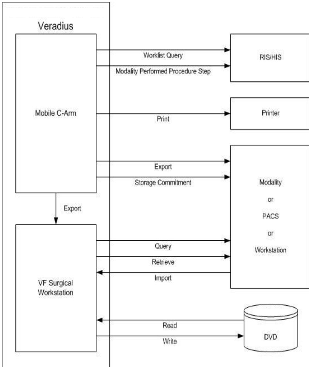
Figure 1: System Overview of Mobile C-Arm with integrated ViewForum Surgical Workstation
