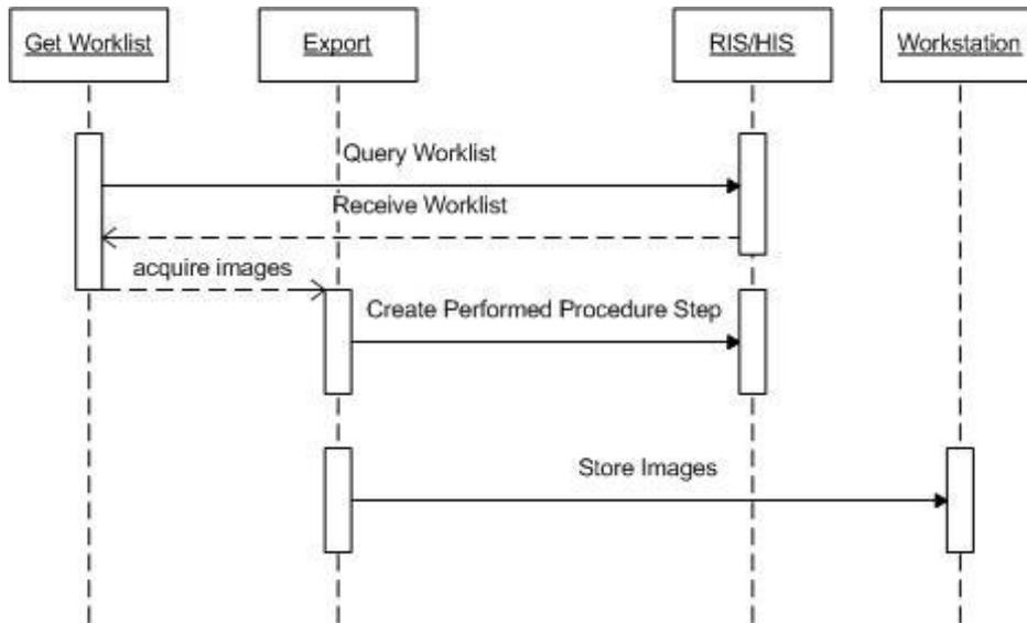
Figure 4: Typical Acquisition Workstation Storage Sequencing Constraint
