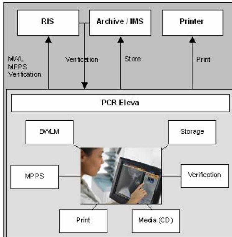
Figure 1: PCR Eleva in a DICOM network
