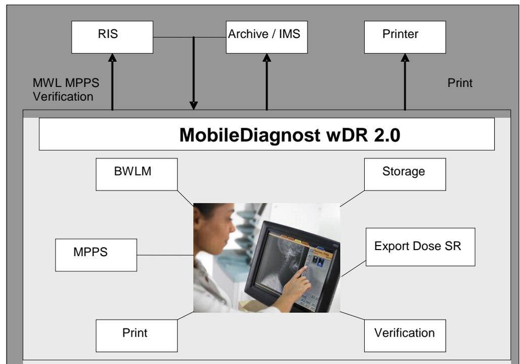
**Figure 1: MobileDiagnost wDR 2.0 in a DICOM network**
