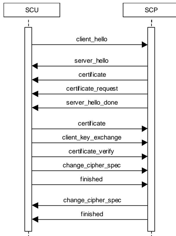
Figure 14: Message flow of TLS handshake
