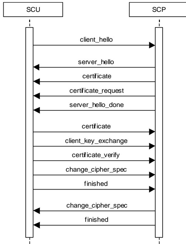
Figure 14 Message flow of TLS handshake
