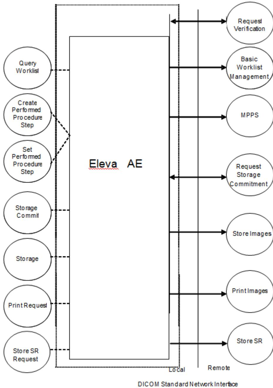
Figure 2 Application Data Flow Diagram
