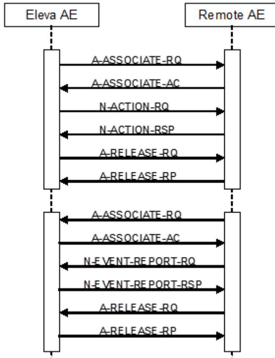
Figure 9 (Real World) Activity – Storage Commitment Push Model as SCU within separate associations (asynchronous)
