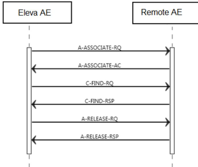
**Figure 12 Data Flow Diagram – FIND as SCU**
