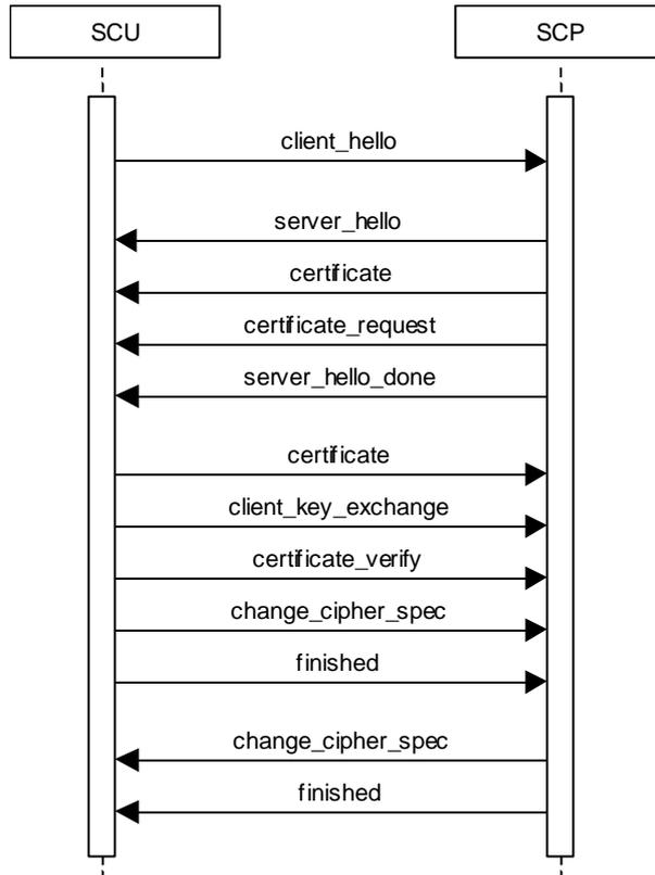
Figure 14: Message flow of TLS handshake
