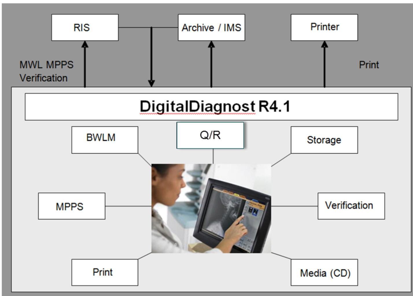
**Figure 1 DigitalDiagnost R4.1 in a DICOM network**
