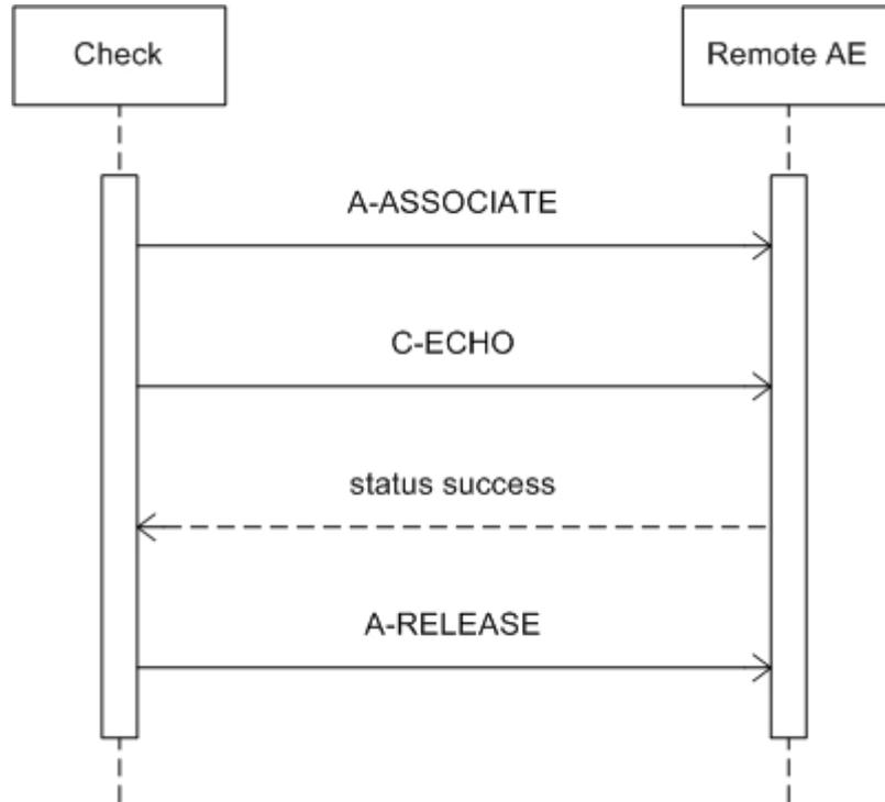
Figure 6: Sequencing of RWA Check
