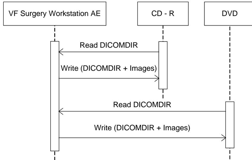
Figure 14: Sequencing of RWA Write Image
