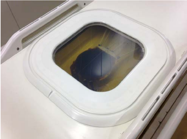
Figure 3. The ultrasonic window of the Sonalleve MR-HIFU system with integrated DISC device .
