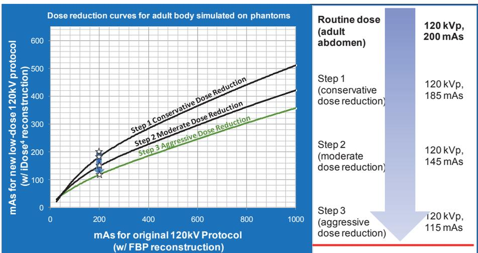
Figure 22: Incremental dose (tube current) reduction steps (for adult phantom using body protocol).
