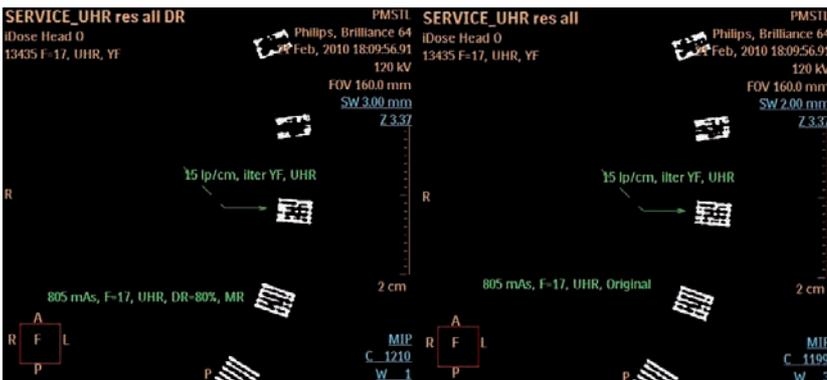
Figure 20: Line-pair phantom demonstrating equivalent spatial-resolution independent of iDose<sup>4</sup> level.
