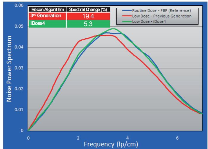
Figure 8: Noise power spectrum (NPS) of 3<sup>rd</sup>- and 4<sup>th</sup> generation reconstruction techniques relative to FBP NPS.
