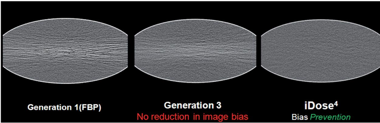
Figure 7: 3<sup>rd</sup>-generation reconstruction (basic iterative reconstruction technique) is unable to remove bias artifacts.
