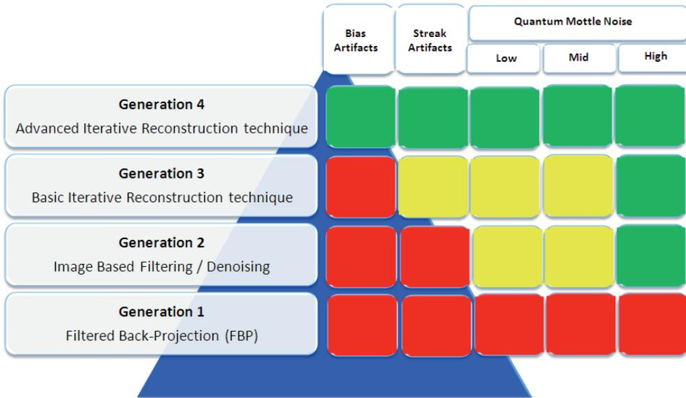
Figure 9: Summary of noise reduction and artifact prevention capabilities provided by each reconstruction generation.
