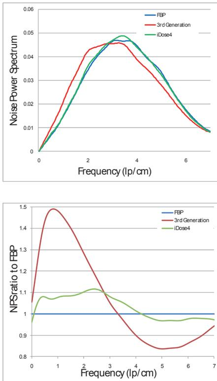
Figure 9: NPS of different reconstruction techniques used for benchmarking (a) original NPS curves (b) NPS ratio to FBP NPS.
