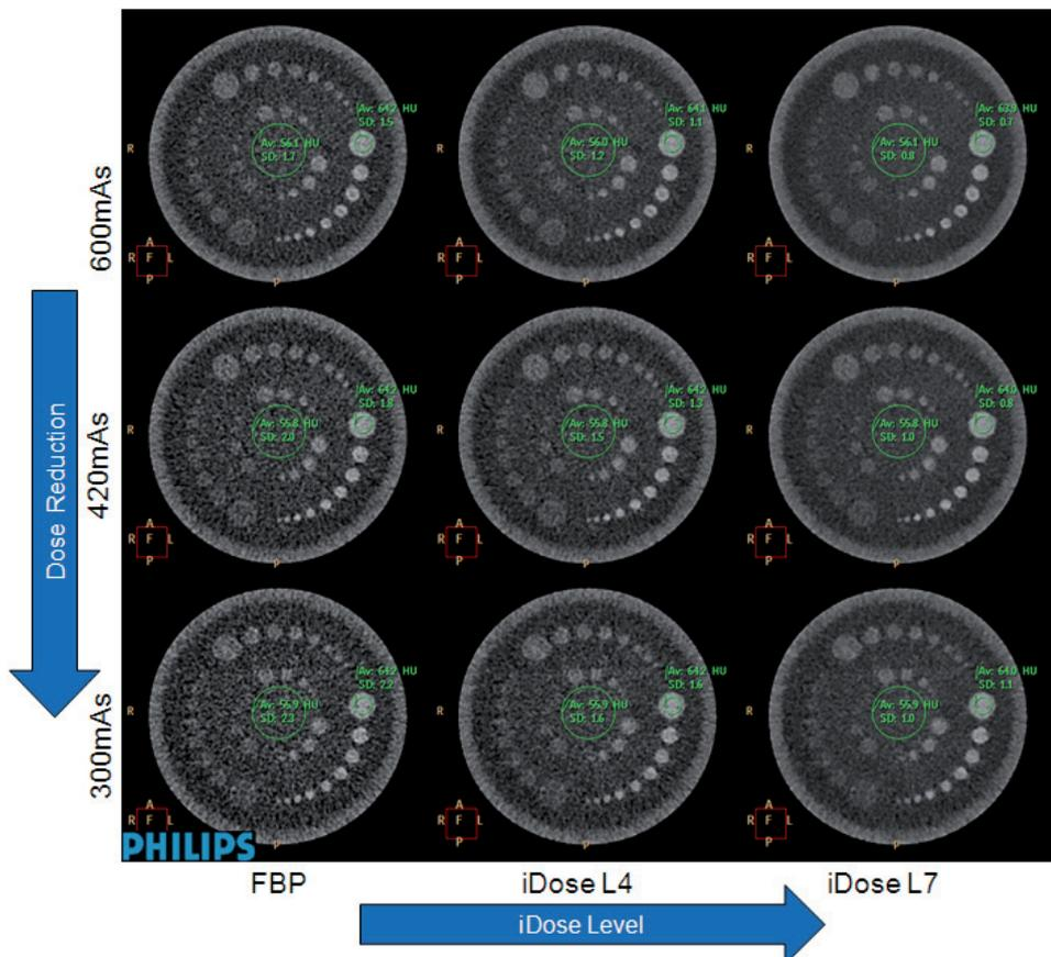
Figure 21: Contrast/Noise Measurements as a function of dose reduction and iDose<sup>4</sup> levels.
