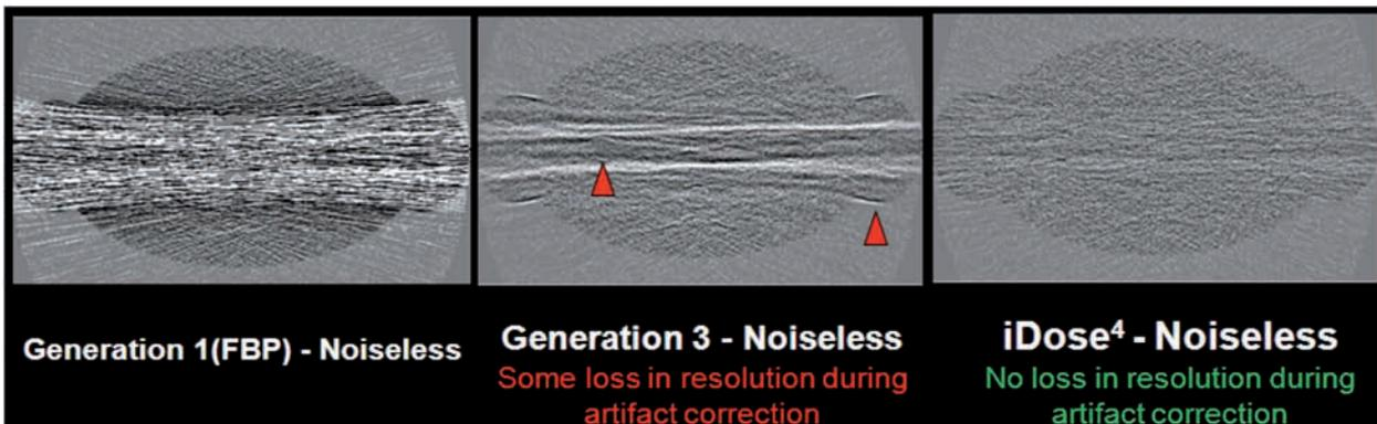
Figure 6: Generation 3 (basic iterative reconstruction technique) result in some loss in resolution.
