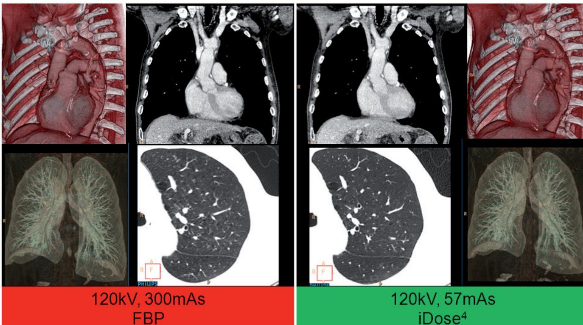
Figure 11: iDose<sup>4</sup> enables up to 80% dose reduction while maintaining diagnostic image quality [Case Courtesy: AsahiKawa Hospital, Japan].
