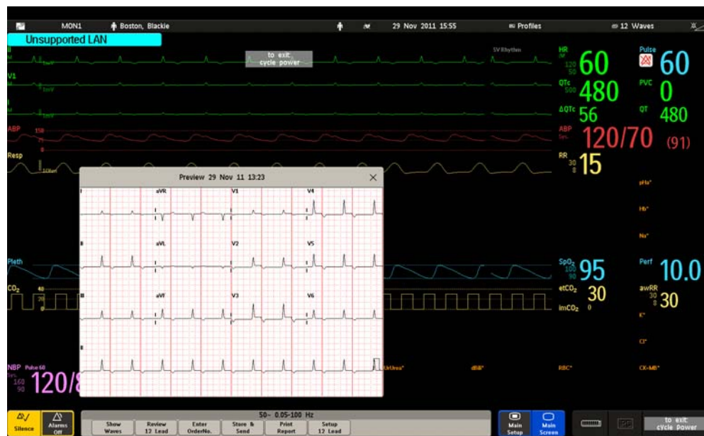
Figure 2: IntelliVue Patient Monitor with 12-lead ECG Application Window open displaying a captured 12-lead Preview
