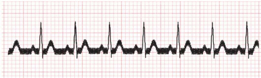
Figure 1-4 Power line interference (50/60 cycles per second)
