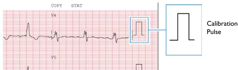
Figure 5-18 Calibration Pulse on the ECG Report
