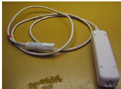
Cable trap used on C1, C3, C4, E1 and R1 coils
