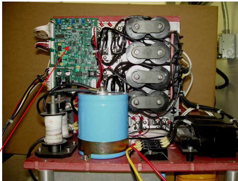
Figure 5 Power Supply – Right Side (Removed From Enclosure For Clarity)
