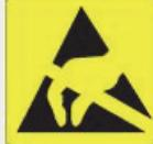
ESD (electrostatic discharge): The product is marked with this symbol to warn the user not to touch exposed pins. Touching exposed pins can cause electrostatic discharge, which can damage the product.
