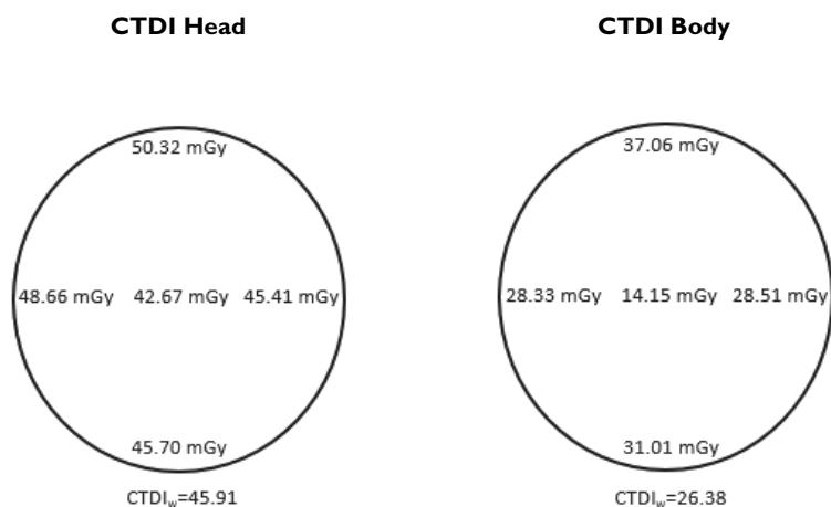
The maximum dose is delivered at the 12 o'clock position on each figure above. The following tables show dosage value (CTDI) of the phantom in different positions (120 kV, 300 mA, 1s,  $32 \times 0.625$  mm) under typical parameter conditions. All measurements are in mGy.
