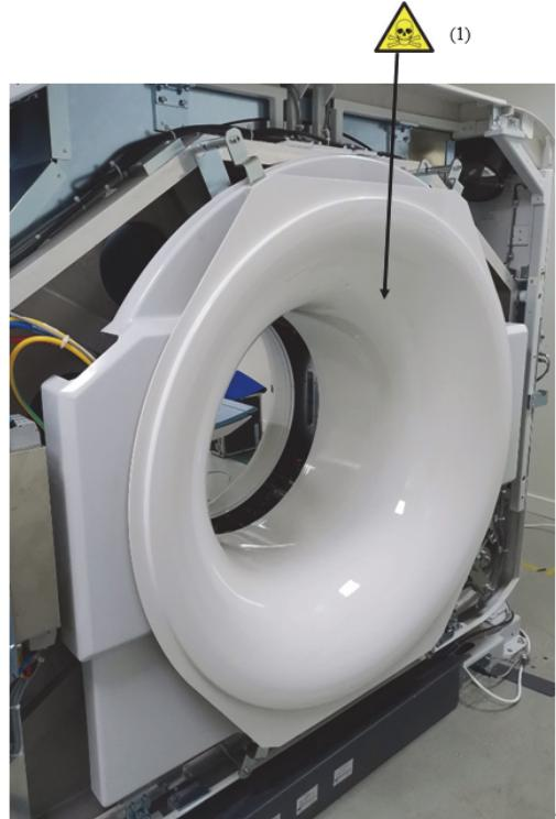
Figure 4: Left Side View of Gantry with Cover Removed
