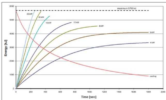
The anode heating and cooling curves show the maximum heat content of the X-ray tube.
