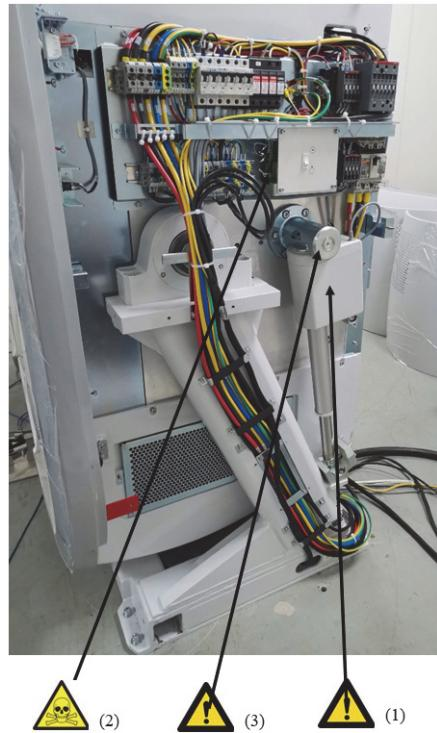
Figure 5: Right Side View of Gantry with Cover Removed
