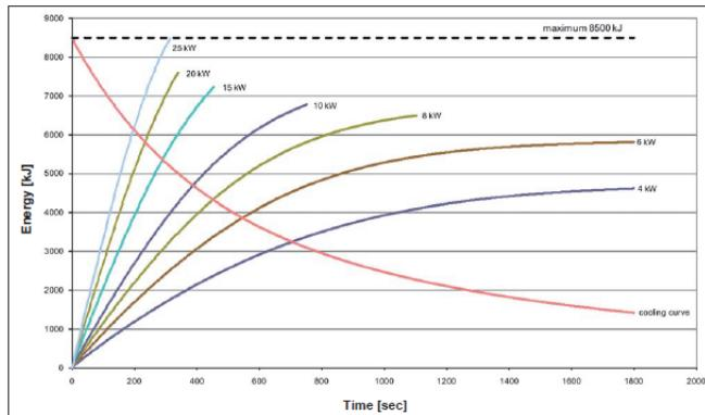
The heating and cooling curves include the heat capacity of the cooling unit. They show the maximum heat content of the X-ray tube assembly.
