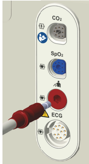
Figure 10 Connecting the NBP Cable
