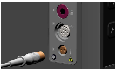
Figure 13 Connecting the Temperature Cable
