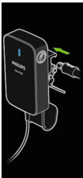
Figure 31 Animated guidance for connecting the pressure wire
