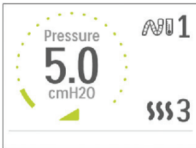
Ramp Pressure Screen
