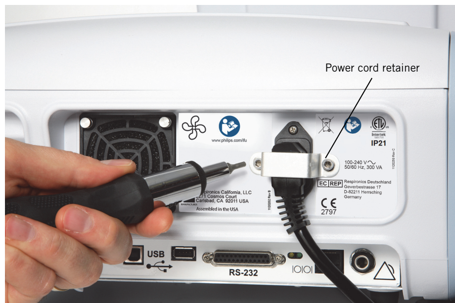
Figure A-5: Installing the power cord retainer
