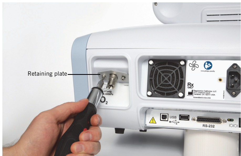
Figure A-4: Installing the oxygen inlet connector
