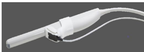
Figure 5: EM Tracker with Probe Holder
