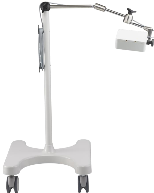
Figure 17: Pole Cart Field Generator Mounting
