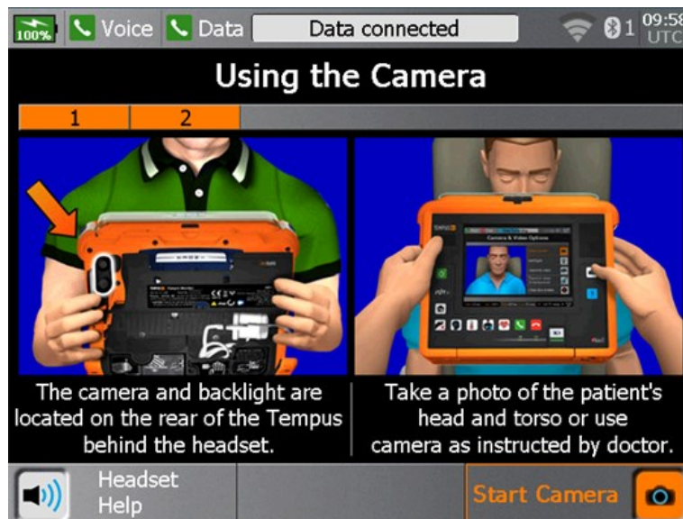
Example of the Tempus IC2 display showing location of the digital picture
