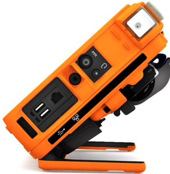
Communications connection panel
