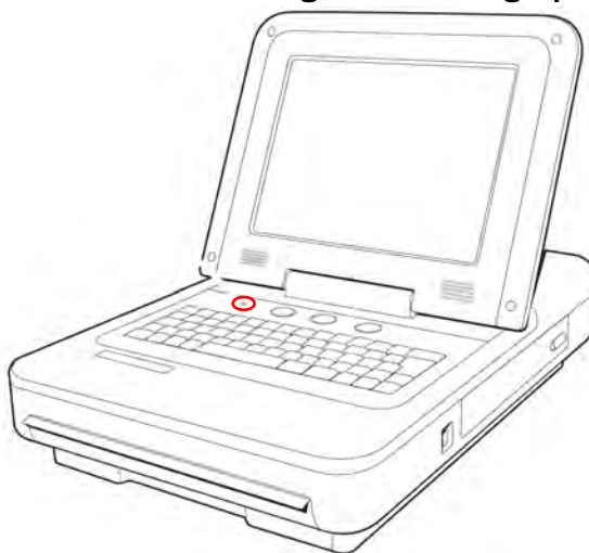
Figure 5-5 AC power on indicator light on cardiograph
