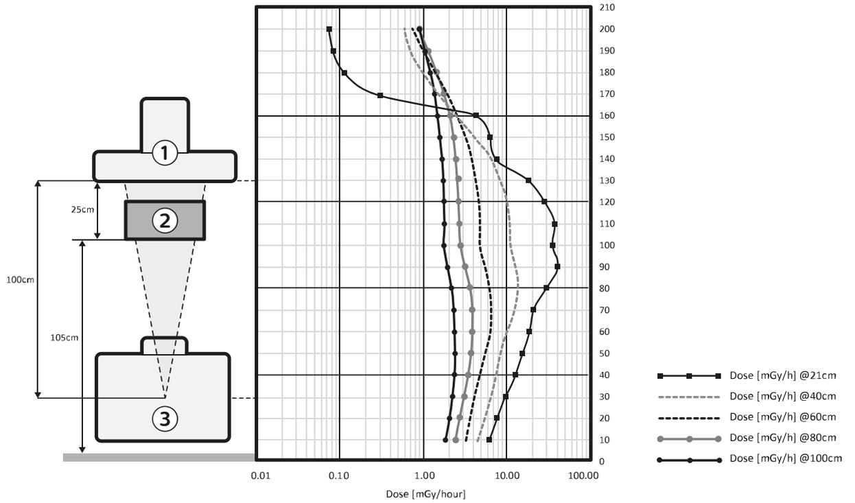
**Figure 141** Designated significant zone of occupancy for FD15
