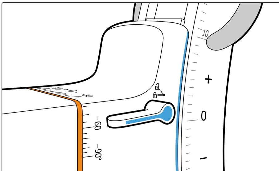
**Figure 44** Angulation brake handle
