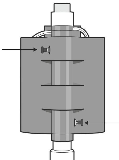
**Figure 39** Monitors: locking bolts for transport
