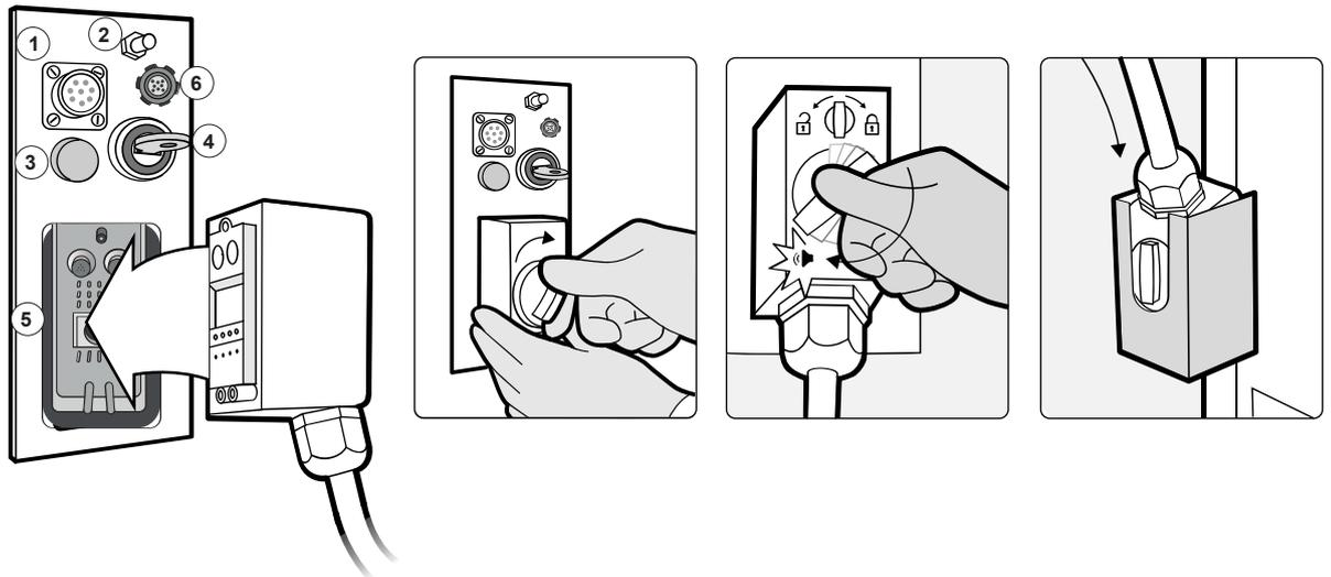
**Figure 48** C-arm stand connector panel with cable connections
