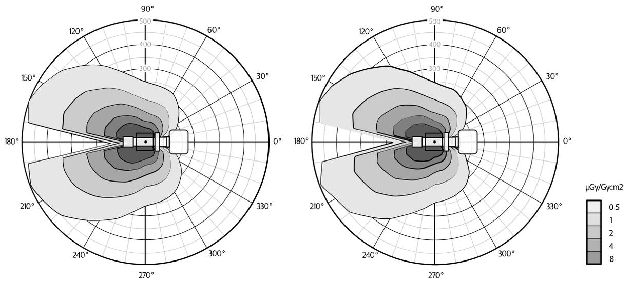
**Figure 150** Isokerma map for FD17, horizontal position, tube at 180 degrees, at 1.0 m (left) and 1.5m (right)
