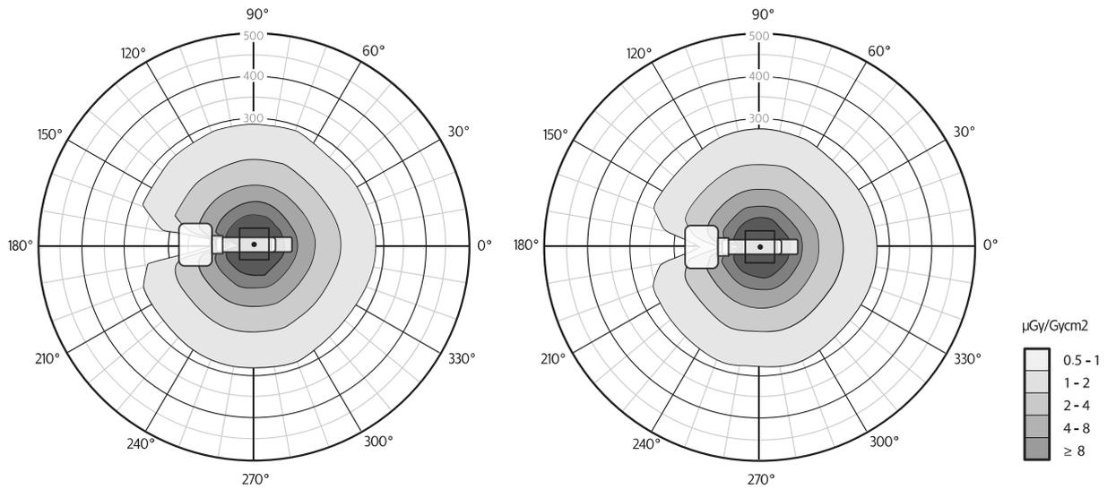
**Figure 149** Isokerma map for FD12, lateral position, tube opposite stand, at 1.0 m (left) and 1.5m (right)
