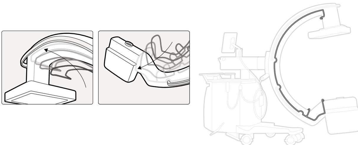
**Figure 113** Fitting the spring bow
