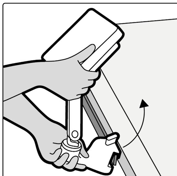
**Figure 116** Detaching the Swing Arm to Accessory Rails
