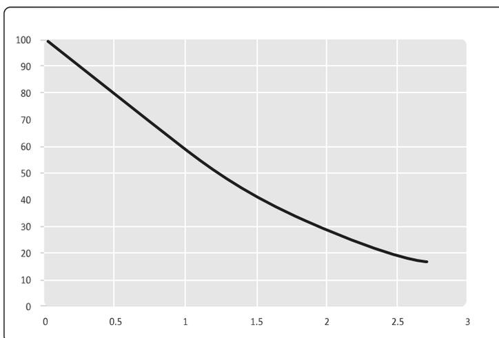
**Figure 136** MTF at 2 Gy / RQA5 exposure according to IEC62220-1-3
