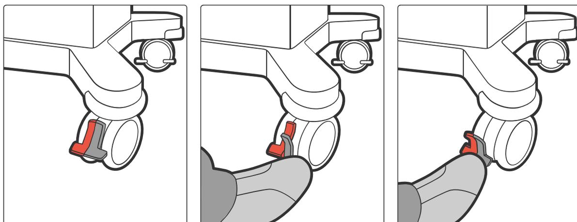
**Figure 37** Wheels unlocked, locked for transportation with brakes not applied, and braked.
