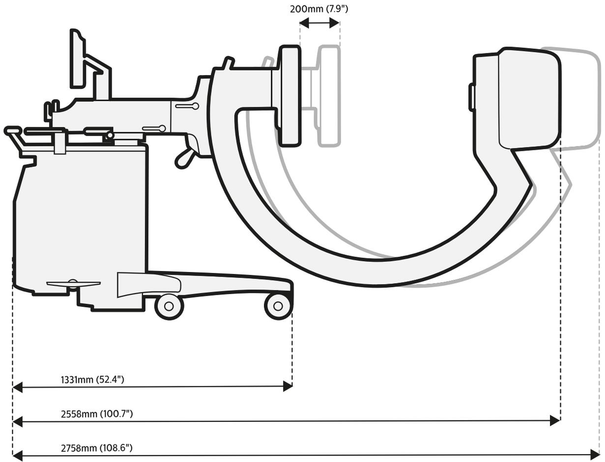
**Figure 152** C-arm stand dimensions: longitudinal movement
