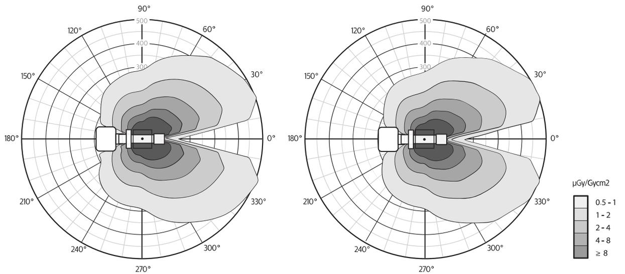
**Figure 146** Isokerma map for FD15, horizontal position, tube opposite stand, at 1.0 m (left) and 1.5m (right)
