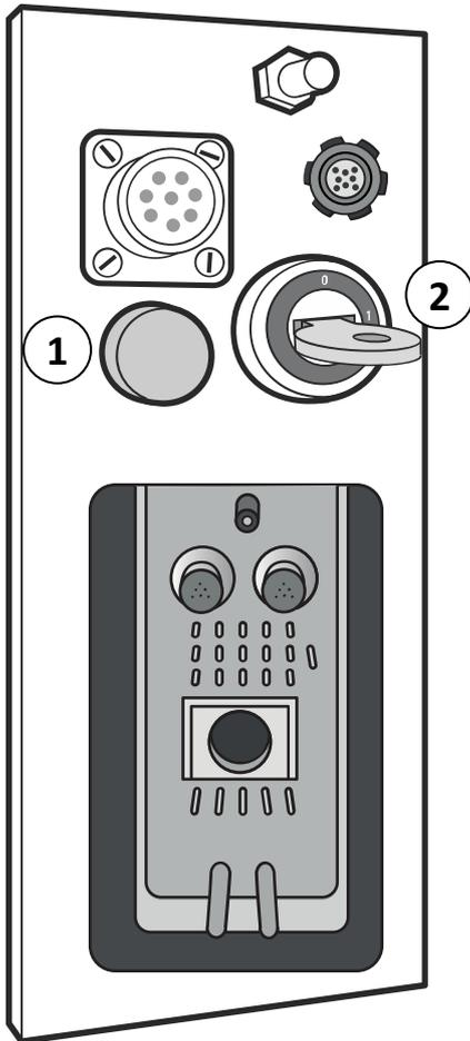
**Figure 55** Energy storage unit charge indication light and system lock
