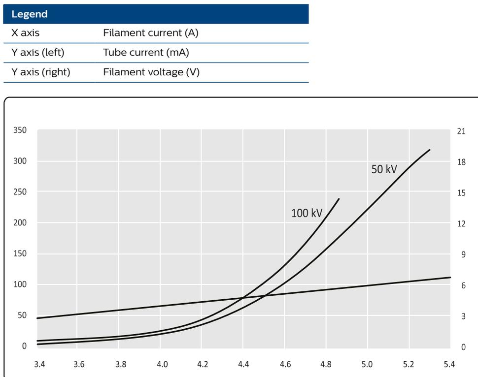
**Figure 130** Emission characteristics large focus
