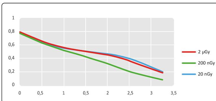
**Figure 137** DQE vs. spatial frequency at 20 nGy / 200 nGy / 2 Gy in RQA5 exposure according to IEC62220-1-3
