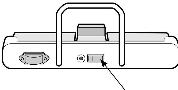
**Figure 112** Wireless foot switch on/off switch
