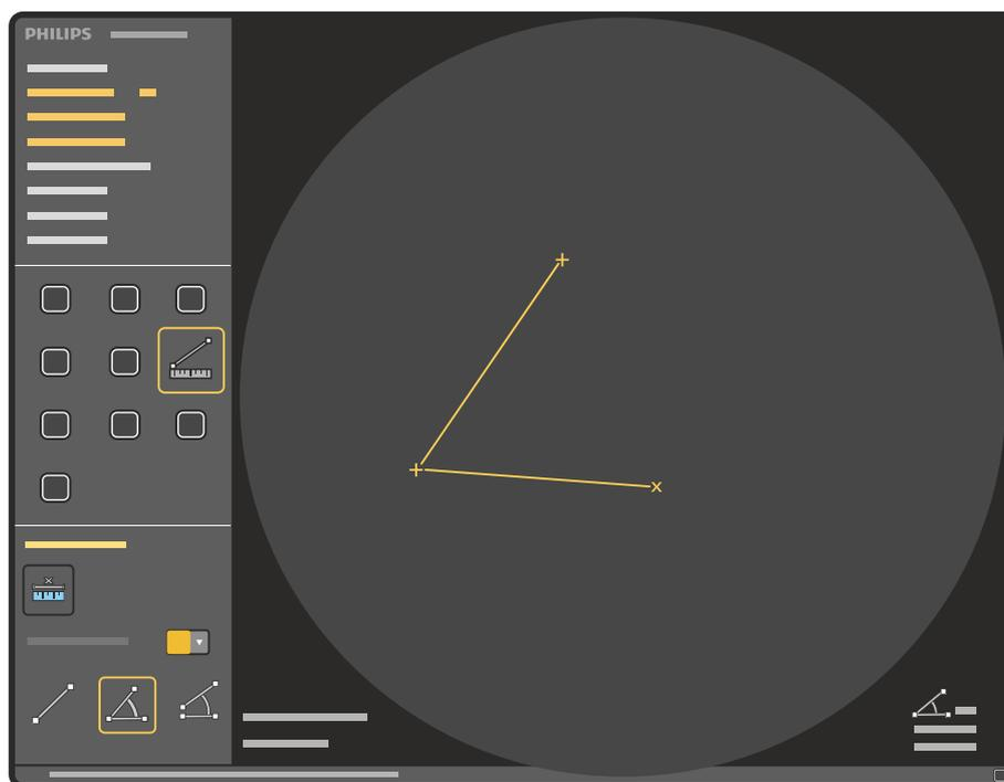
**Figure 87** Measurement of two distances and angle (three points)
