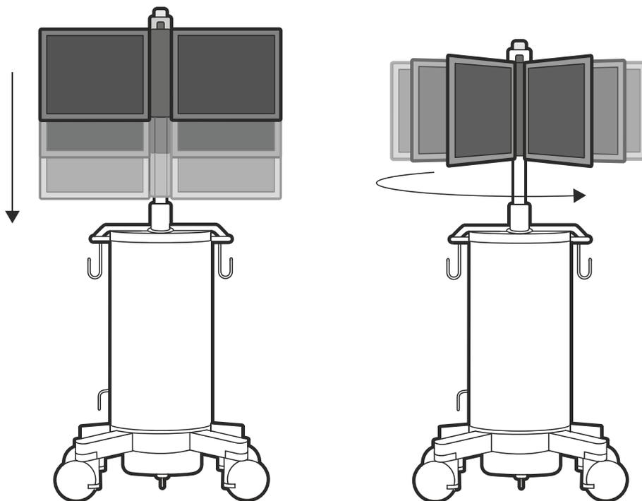
**Figure 56** Monitors: height (left) and swing (right) movements
