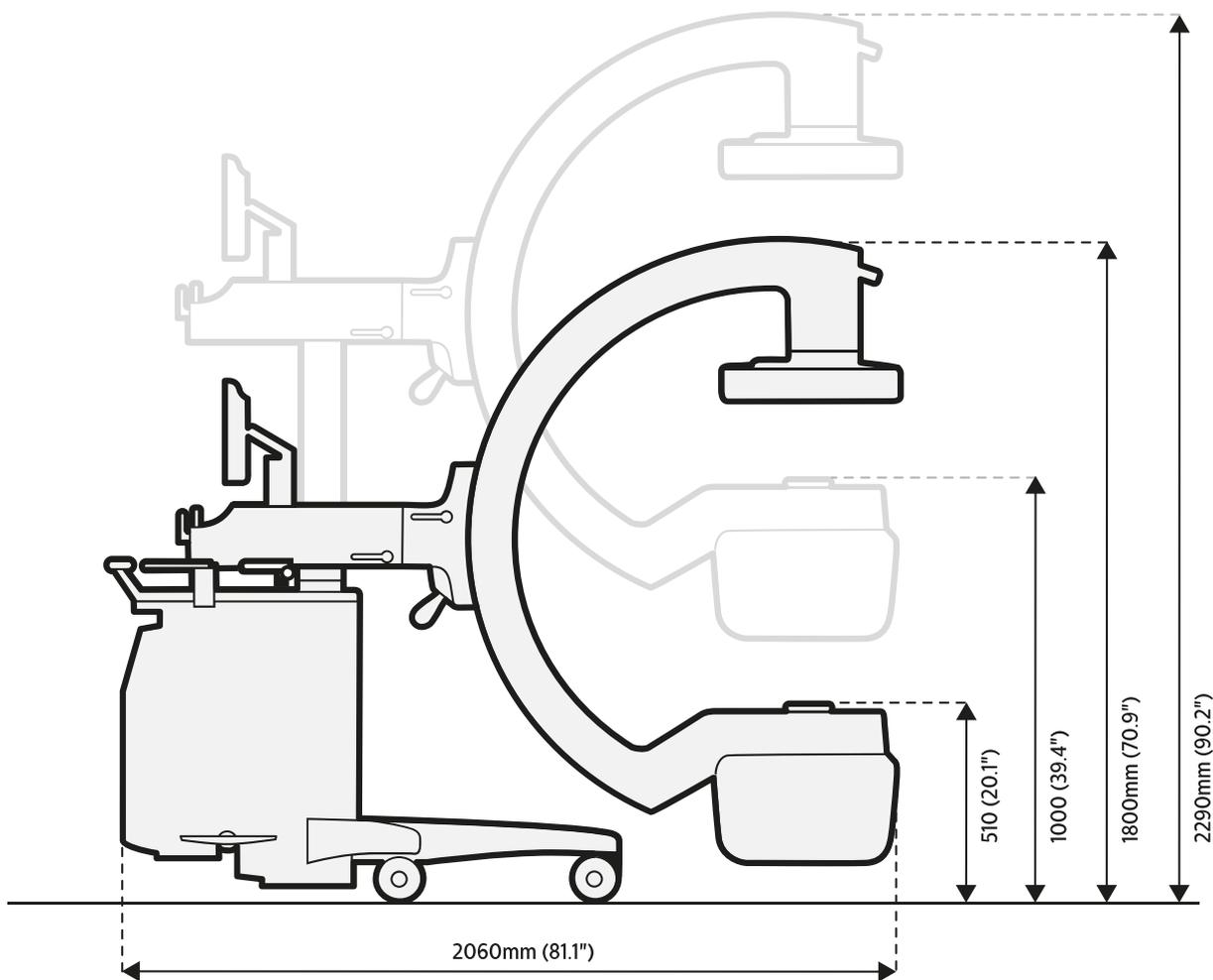
**Figure 153** C-arm stand dimensions: height movement
