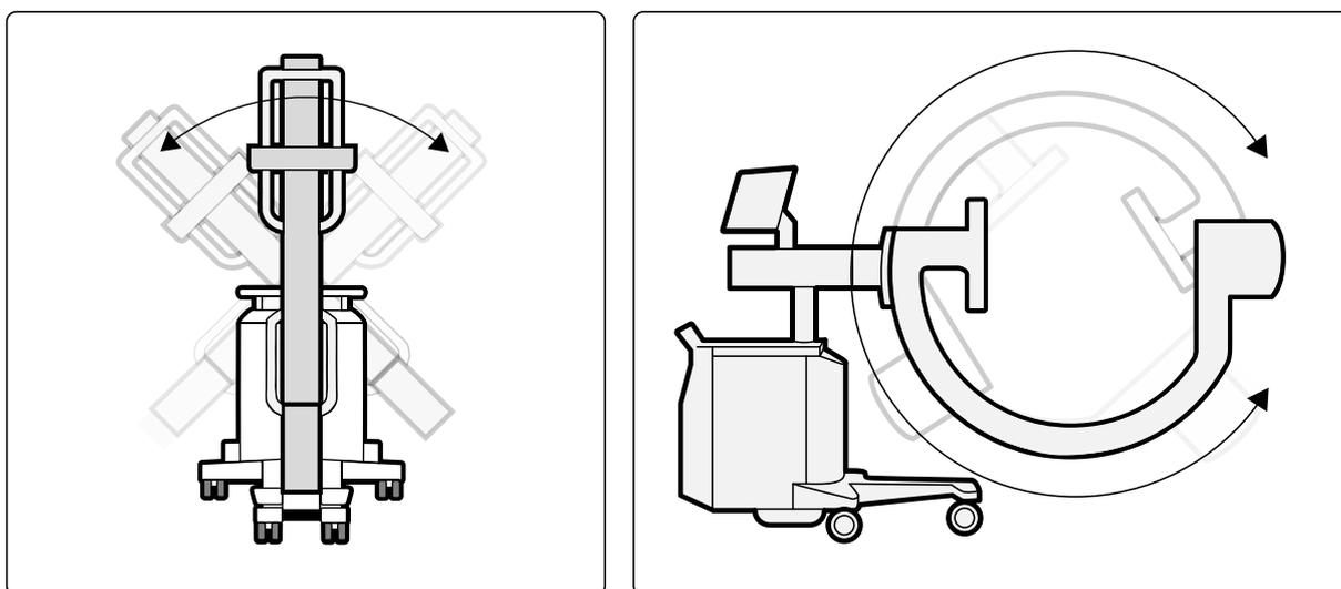
**Figure 17** C-arm rotation (left) and angulation (right)
