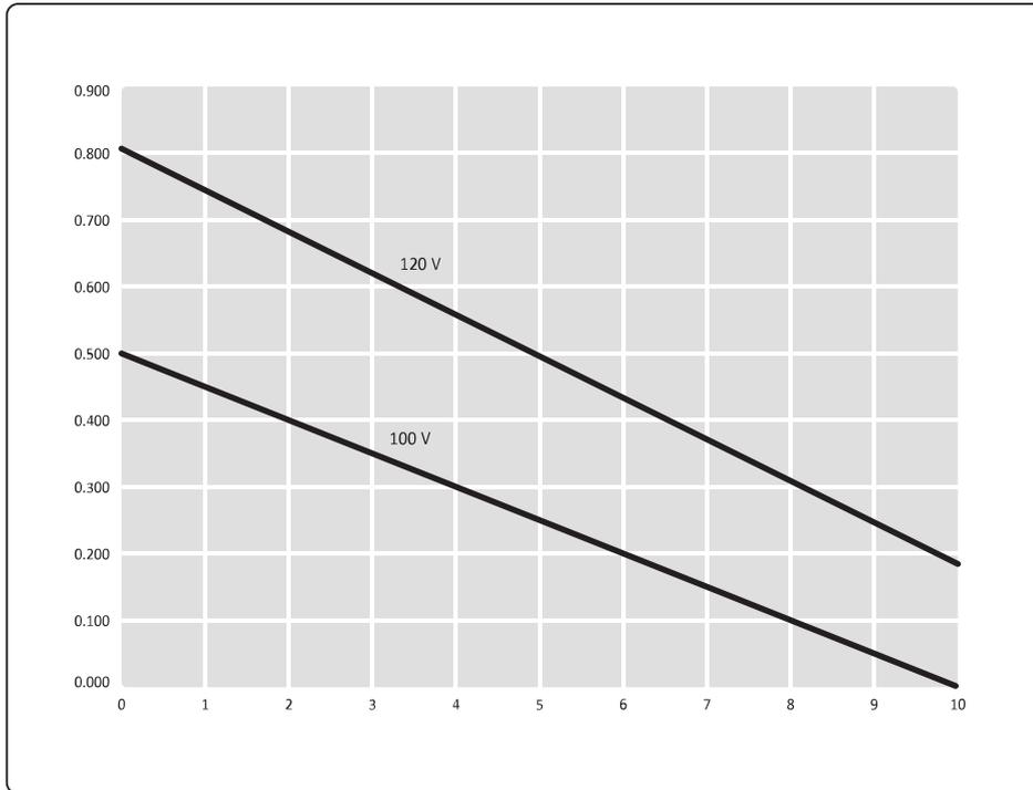
**Figure 158** Maximum mains resistance versus main voltage tolerance
