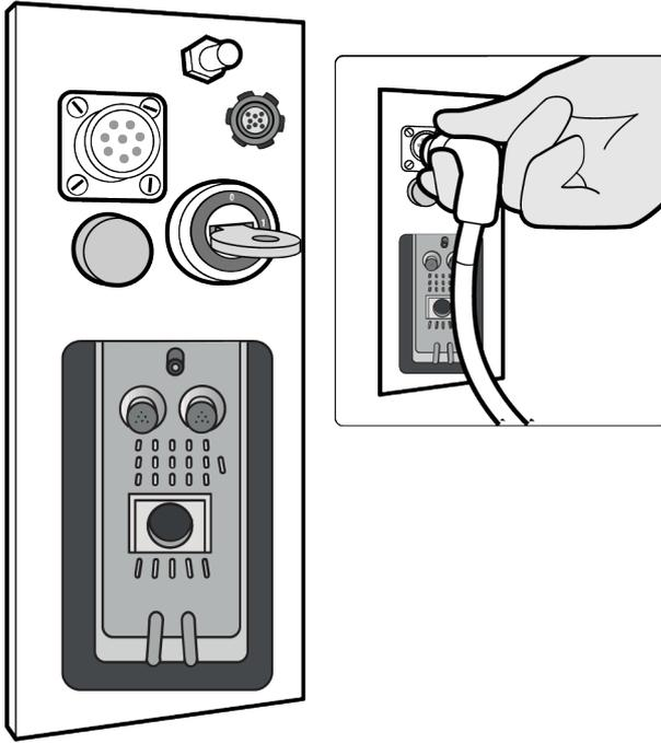
**Figure 125** Connecting the wired foot switch to the C-arm stand
