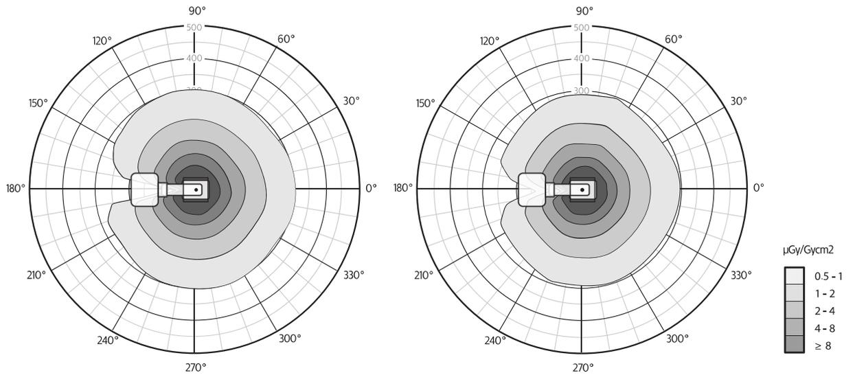
**Figure 147** Isokerma map for FD15, lateral position, tube opposite stand, at 1.0 m (left) and 1.5m (right)
