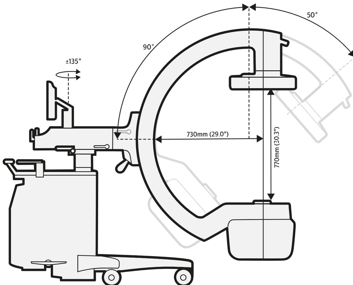
**Figure 154** C-arm stand dimensions: angulation
