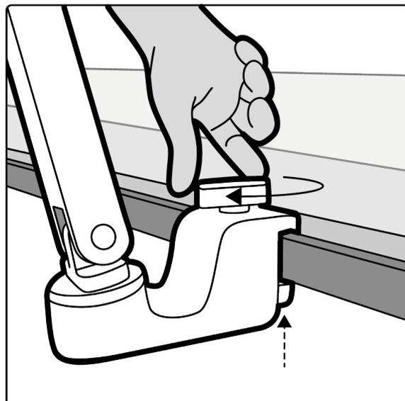
**Figure 115** Attaching the Swing Arm to Accessory Rails
