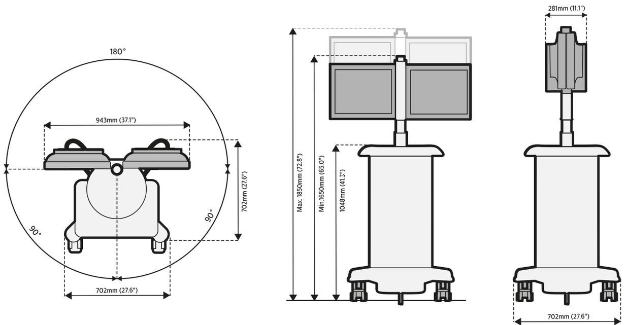
**Figure 157** Mobile view station dimensions
