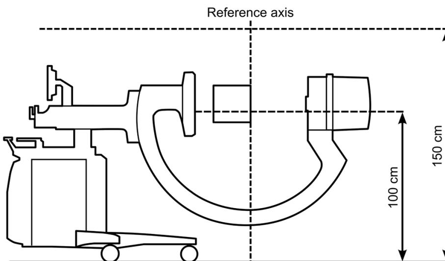
**Figure 144** Isokerma map measurement configuration (horizontal)
