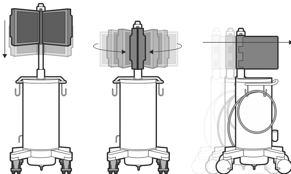
**Figure 38** Putting the monitors in the transport position
