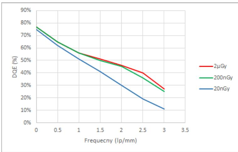
**Figure 139** DQE vs. spatial frequency at 20 nGy / 200 nGy / 2 Gy in RQA5 exposure according to IEC62220-1-3
