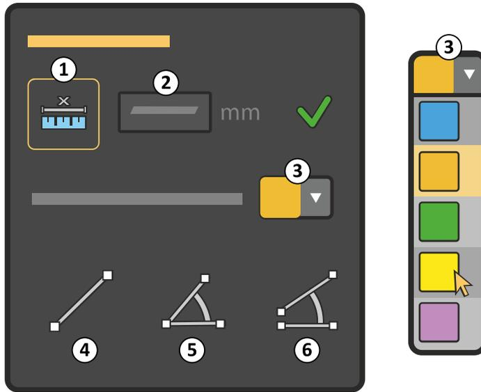
**Figure 85** Measure control panel
