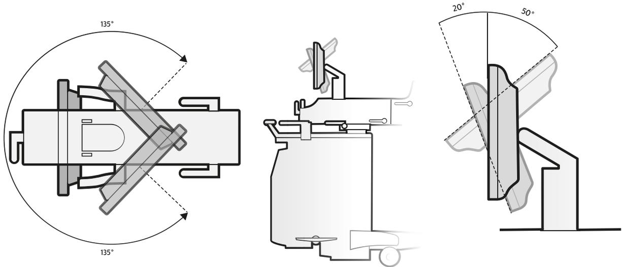
**Figure 156** Stand monitor: rotation (left) and tilt (right)
