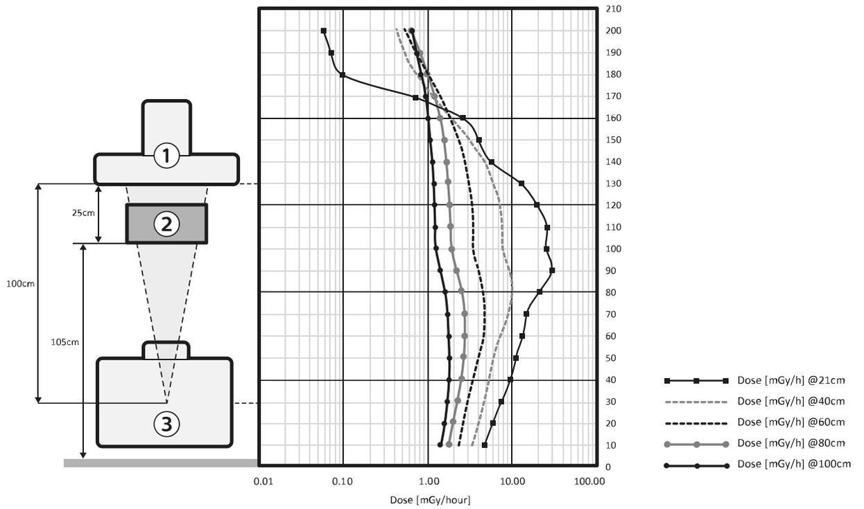
**Figure 142** Designated significant zone of occupancy for FD12
