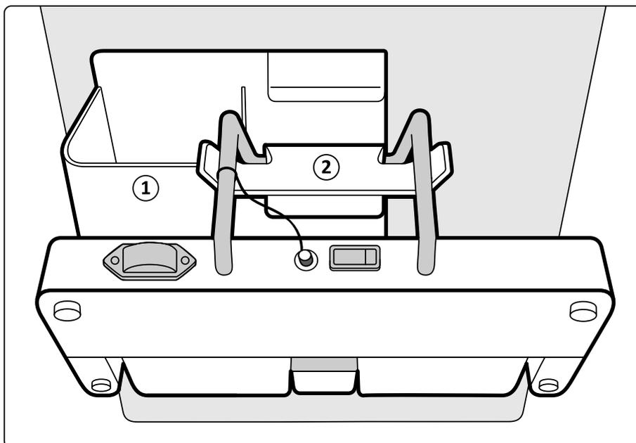
**Figure 111** Wireless foot switch and charger storage on the mobile view station
