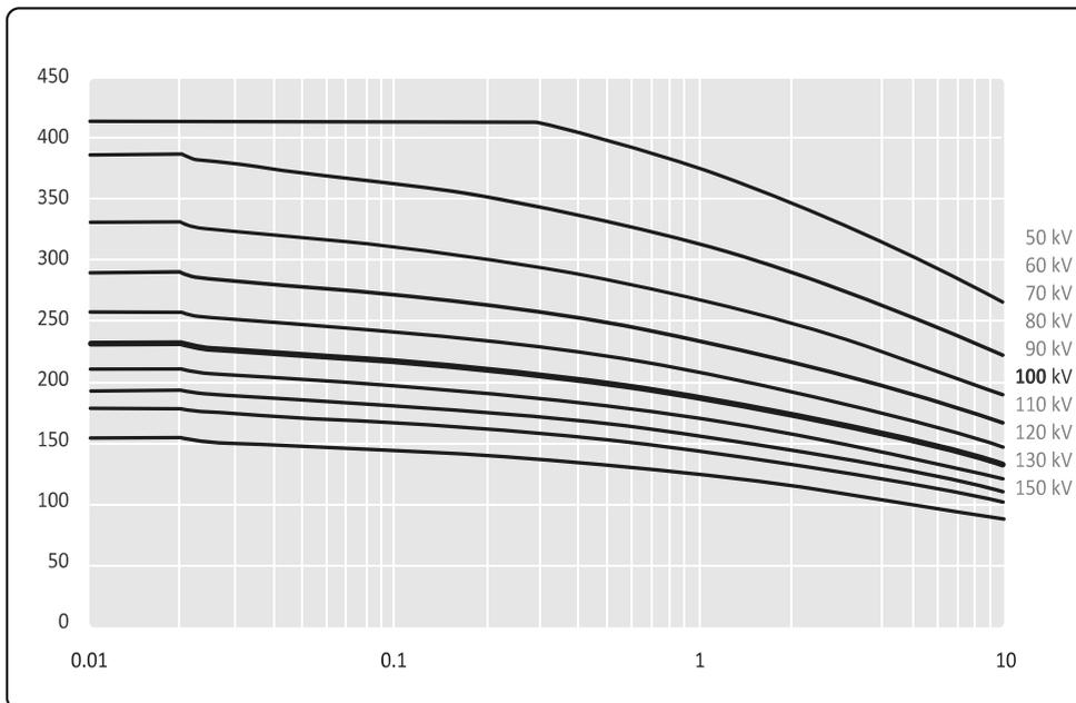
**Figure 132** Single load rating large focus (40% anode heat content)
