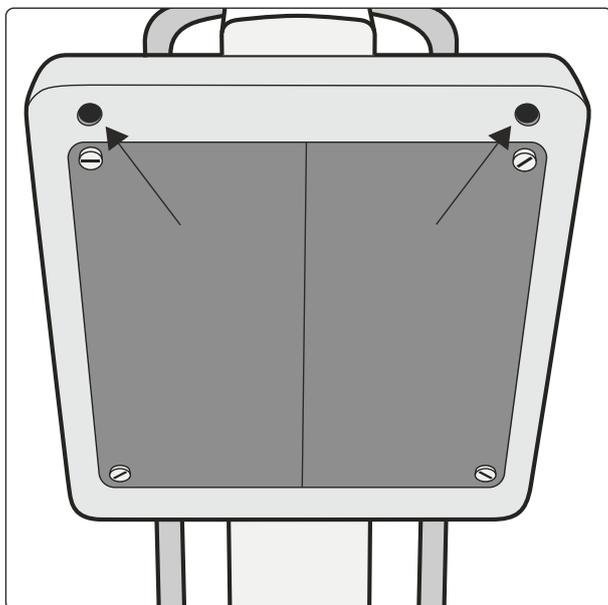
**Figure 26** Detector laser aiming device
