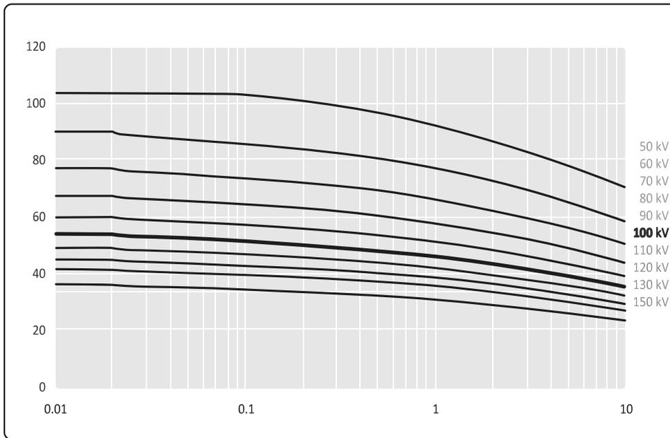
**Figure 131** Single load rating small focus (40% anode heat content)
