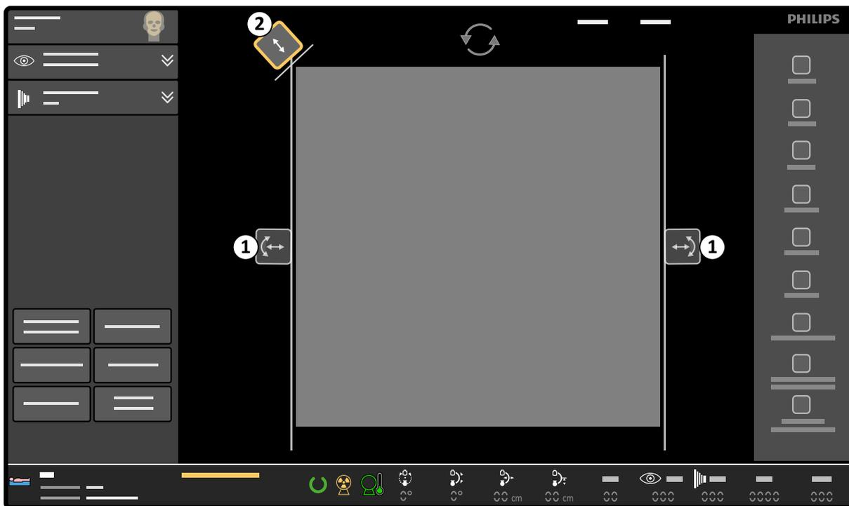
**Figure 66** Collimator and shutter controls on the C-arm stand touch screen
