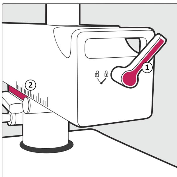
**Figure 45** Longitudinal brake handle and movement measurement
