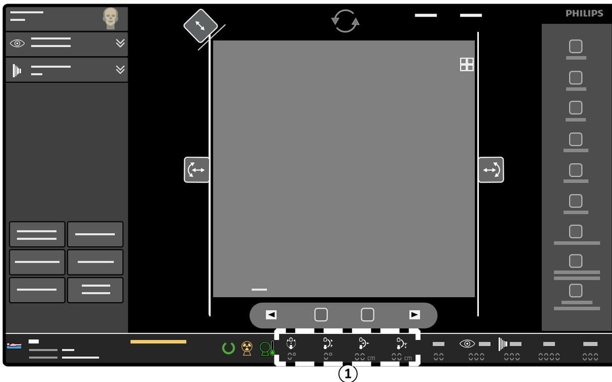
**Figure 99** Position tracking in the C-arm stand touch screen status area (1)
