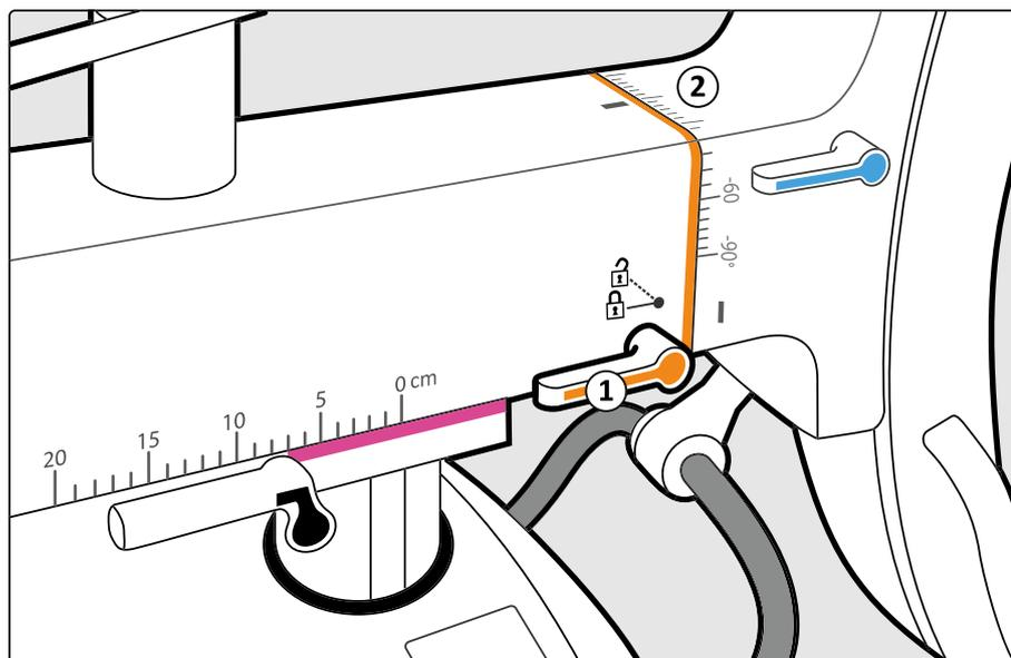
**Figure 43** Rotation brake handle and degrees of rotation markers
