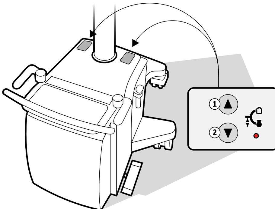
**Figure 162** C-arm stand height movement controls
