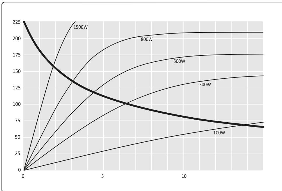
**Figure 128** Anode heating and cooling curves
