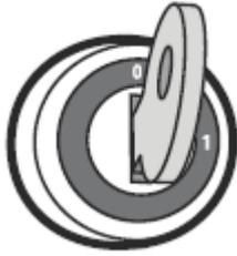
**Figure 3** System lock (system disabled)
