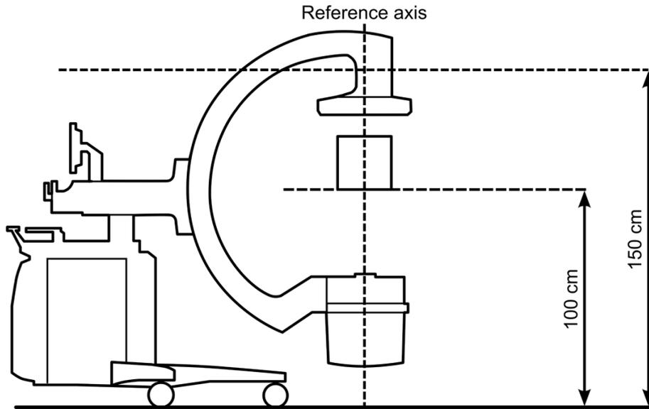
**Figure 145** Isokerma map measurement configuration (lateral)
