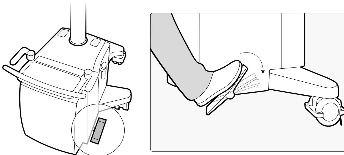
**Figure 34** Releasing the C-arm stand brake
