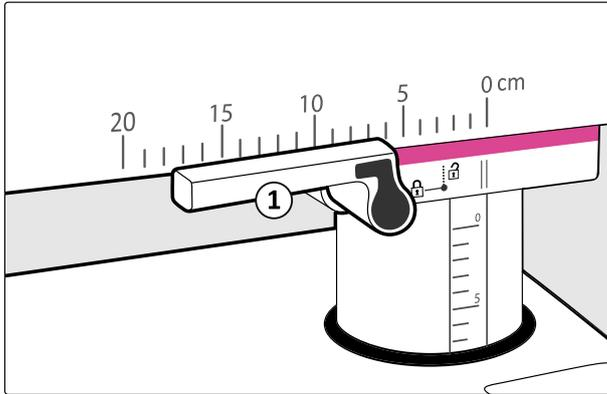
**Figure 46** Swivel (wig-wag) brake handle (1), one handle on each side
