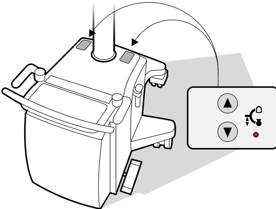
**Figure 47** Height movement buttons
