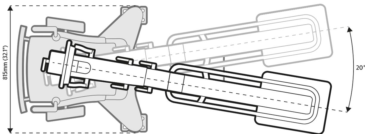
**Figure 155** C-arm stand dimensions: panning movement (swivel)
