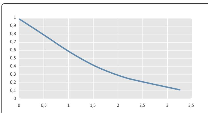
**Figure 138** MTF at 2 Gy / RQA5 exposure according to IEC62220-1-3
