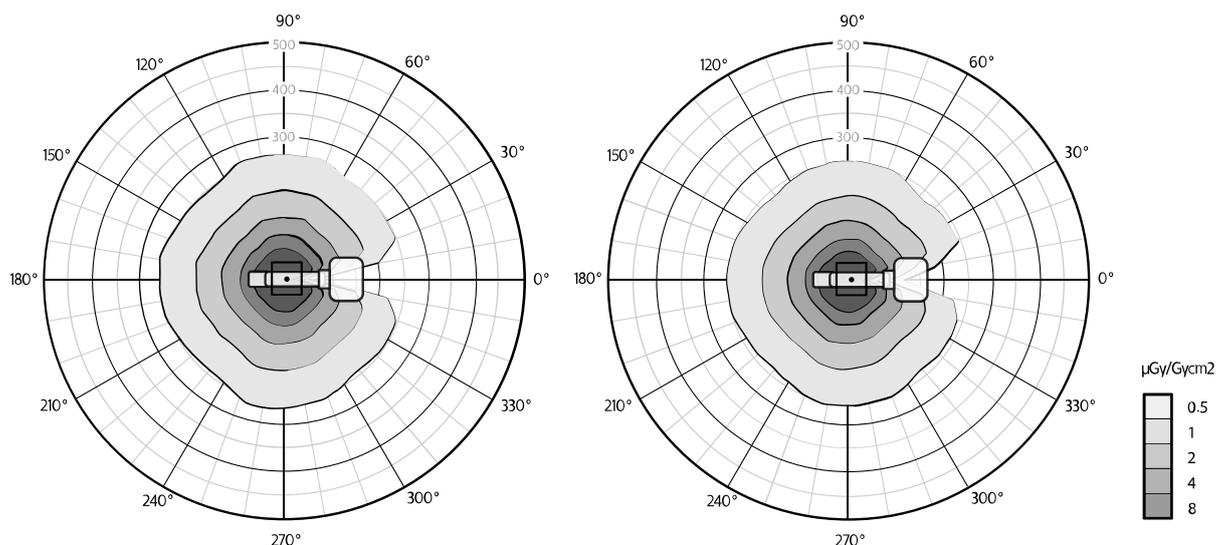
**Figure 151** Isokerma map for FD17, vertical position, tube below, at 1.0 m (left) and 1.5m (right)
