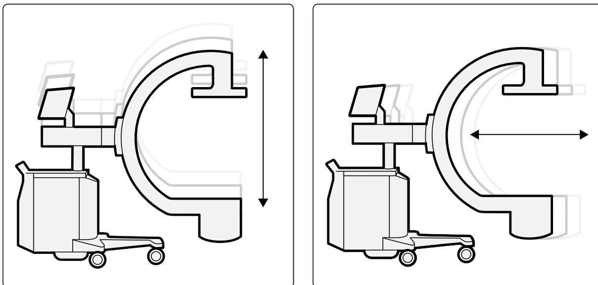
**Figure 18** C-arm height (left) and longitudinal (right) movement
