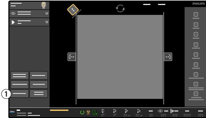
Figure 67 kV Manual button (1) on the C-arm stand touch screen
