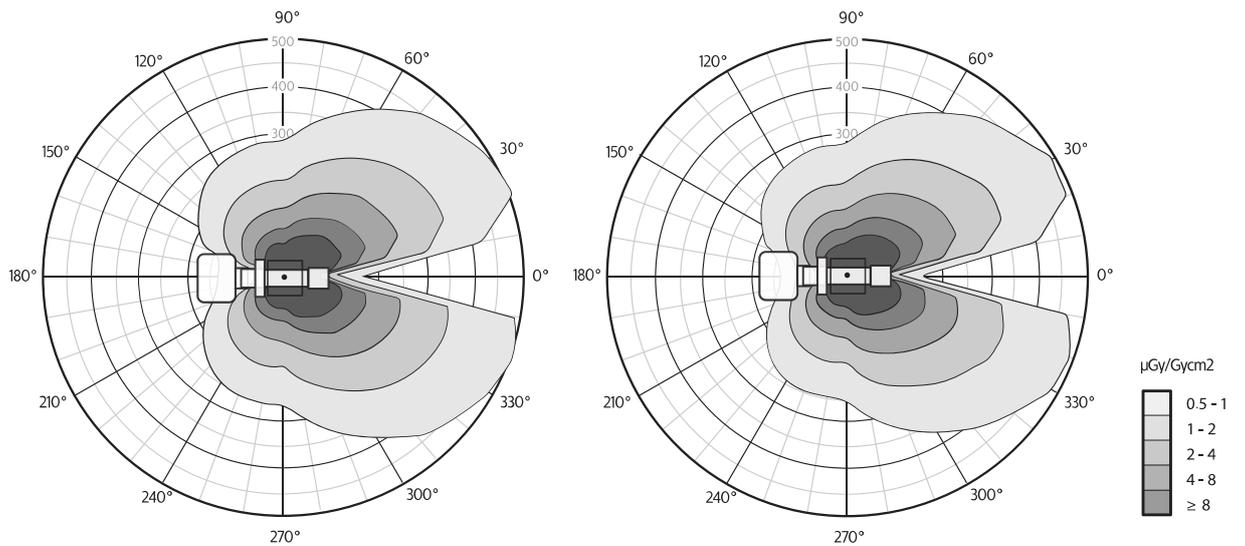
**Figure 148** Isokerma map for FD12, horizontal position, tube opposite stand, at 1.0 m (left) and 1.5m (right)
