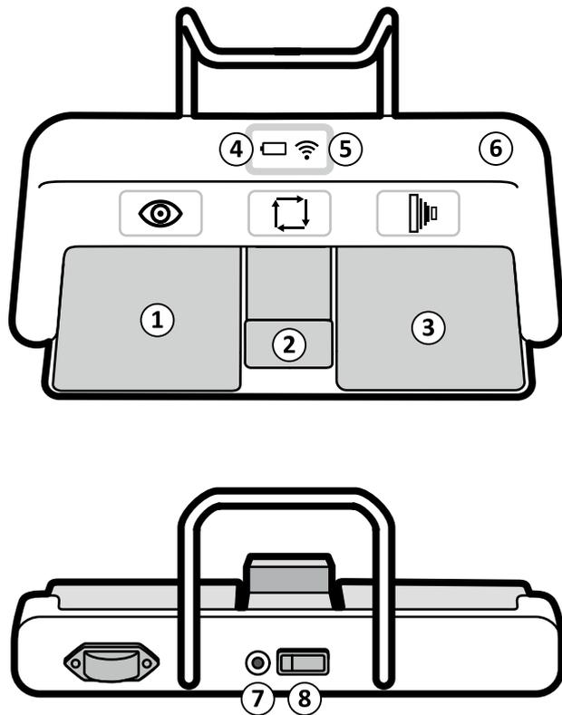
**Figure 165** Wireless foot switch
