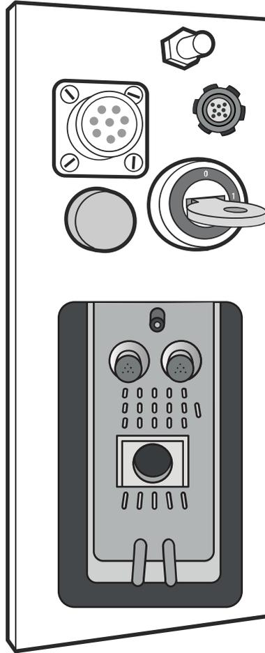
**Figure 118** C-arm stand connector panel
