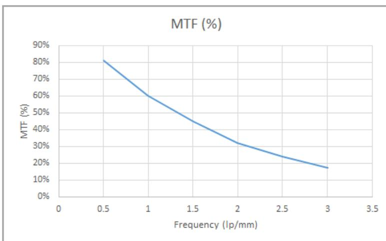
**Figure 140** MTF at 2 Gy / RQA5 exposure according to IEC62220-1-3
