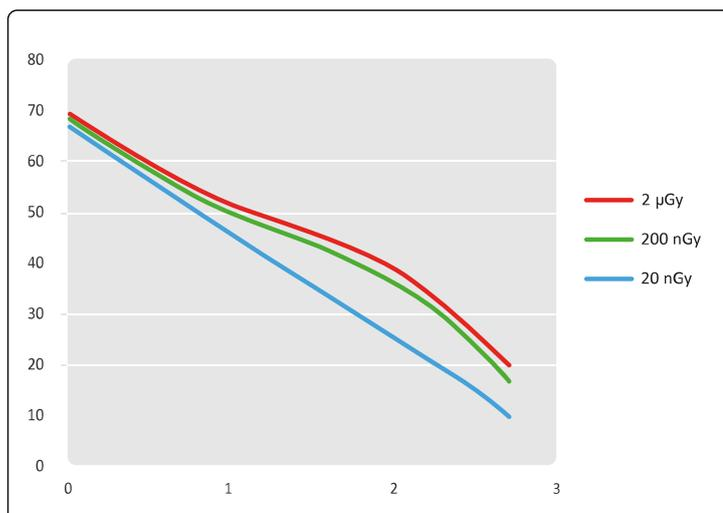
**Figure 135** DQE vs. spatial frequency at 20 nGy / 200 nGy / 2 Gy in RQA5 exposure according to IEC62220-1-3
