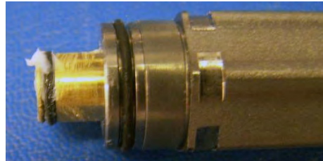
Incorrect: too much lubricant on the o-ring
