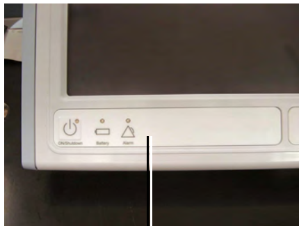
Power switch overlay position on front bezel
