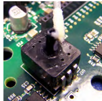
Incorrect: too much lubricant on the sensor stem
