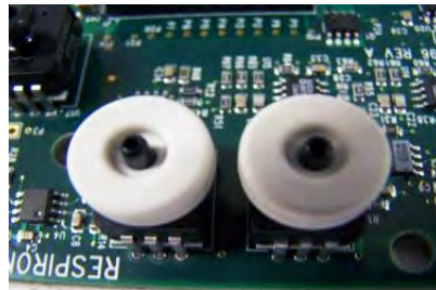
Incorrect: grommets upside down
