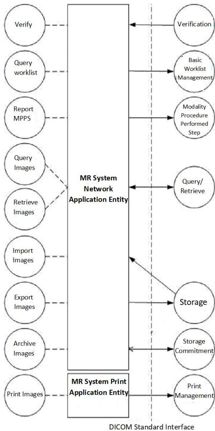
Figure 2: MR System AE Data Flow Diagram
