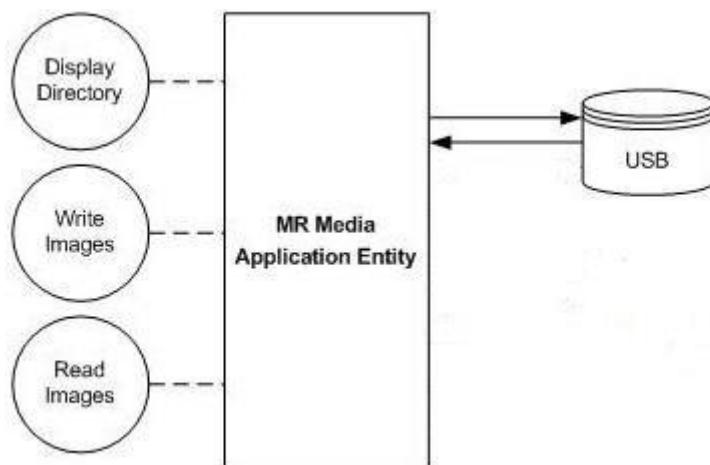
**Figure 18: Media Interchange Application Data Flow Diagram**
