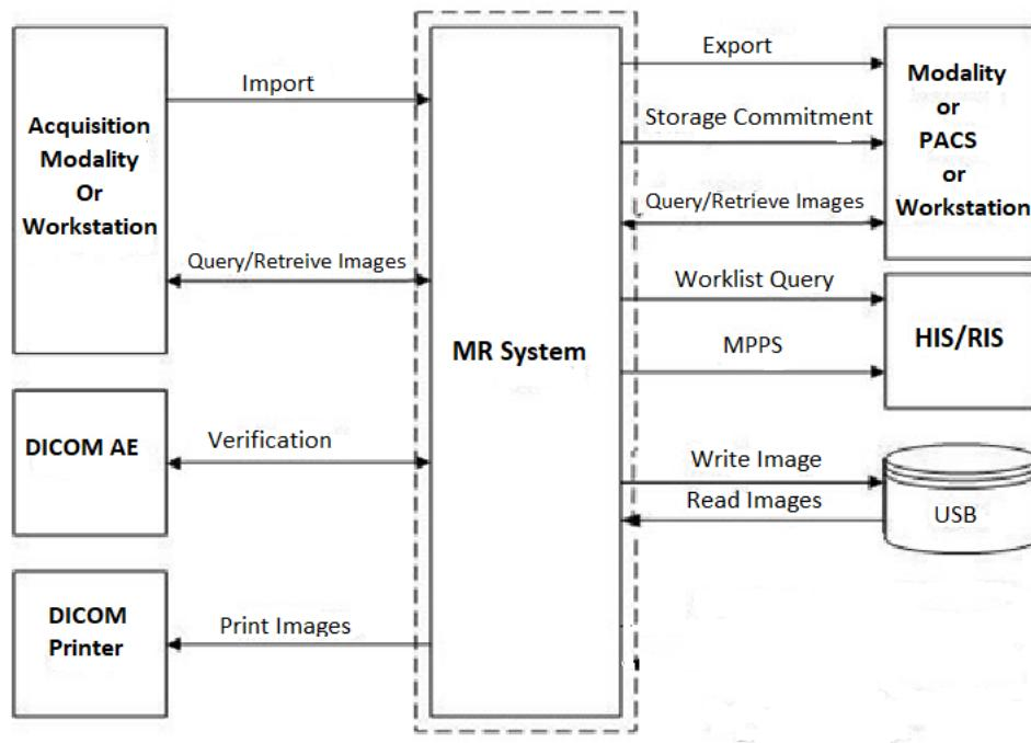
Figure 1: MR System in a DICOM network overview
