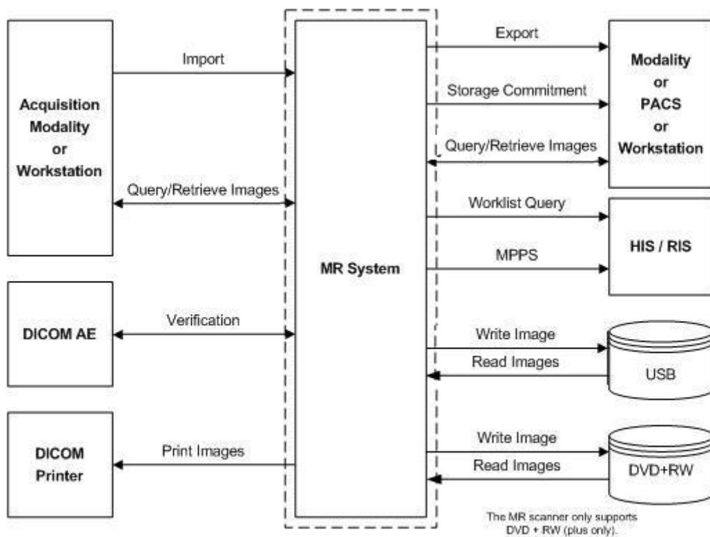
Figure 1: MR System in a DICOM network overview
