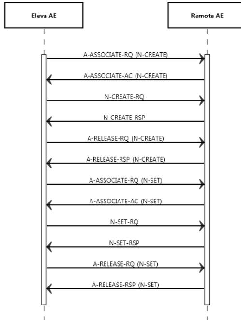
Figure 7: Modality Performed Procedure Step as SCU
