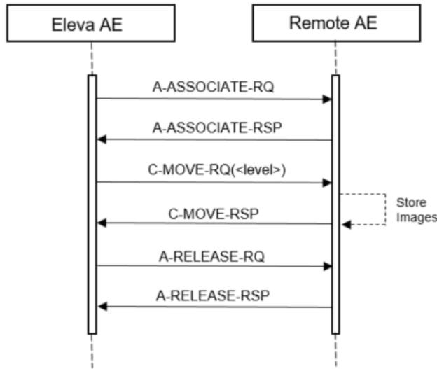
Figure 13: Data Flow Diagram – MOVE as SCU
