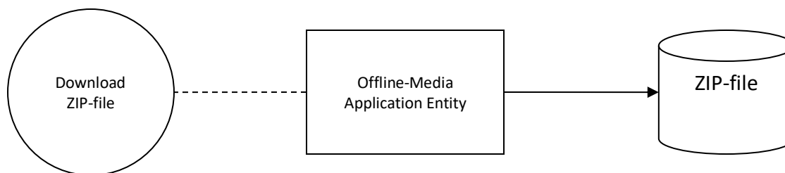
Figure 6 - Application Data Flow Diagram for Media Storage
