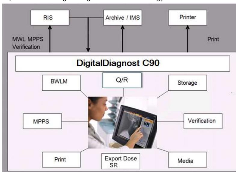
**Figure 1: DigitalDiagnost C90 in a DICOM network**
