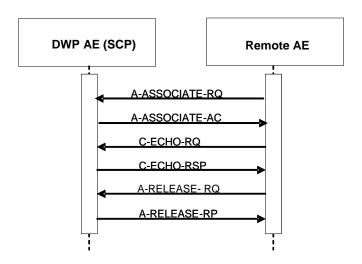
Figure 3: Data Flow Diagram Verification as SCP
