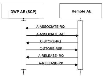
Figure 5: Data Flow Diagram Image Import.
