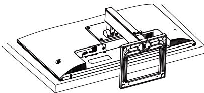
2. Loosen the assembly screws, then detach the neck from the monitor.
