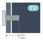
50"/55"/65" 300x300mm Upper: M6 (L: 20.5mm ~ 32mm) Lower: ST6 (L: 8mm ~ 11.5mm)
