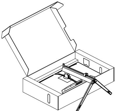
2. While keeping the release button pressed, tilt the stand and slide it out.
