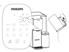
(4) When the " ⟨x" light flashes, you will hear 3 beeps. Empty the water in the tap water tank, refill it with fresh tap water up to the Max line, and place it back.
