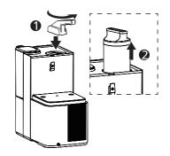
(3) Insert the new filter cartridge into the filter cartridge holder and rotate it clockwise to the locked " (19 machine) position, and cover the machine top lid. Put the tap water tank back to the dispenser.
