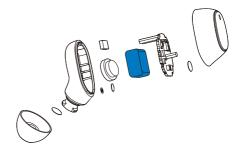
Make sure the charging box is disconnected from the USB charging cable before removing the battery.
