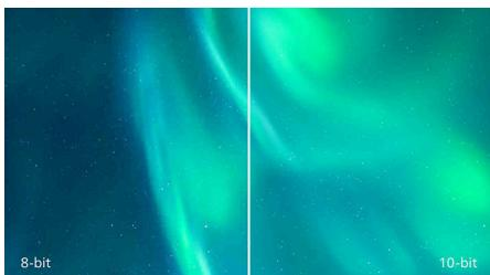
The 10-bit display delivers rich color depth with 1.07 billion colors and 12-bit internal processing for re-creating smooth, natural colors without gradations and color banding.
