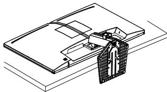
2. While keeping the release button pressed, tilt the stand and slide it out.
