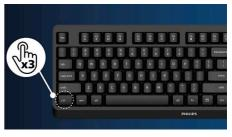
Unlike traditional built-in KVM monitor button, the smart KVM allows for switching between sources with the click of a button on your keyboard. When all devices are properly connected, users can easily switch between sources by clicking the "Ctrl" key three times.
