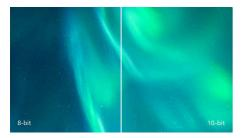
The 10-bit display delivers rich color depth with 1.07 billion colors and 12-bit internal processing for re-creating smooth, natural colors without gradations and color banding.
