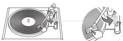
2 Lower the lift lever, and lock the tone arm clip to fix it.
