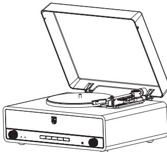
2 Lift up the dust cover vertically from the hinge base.
