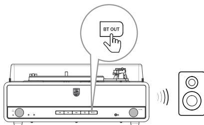
2 Ensure your Bluetooth enabled device is in pairing mode.
