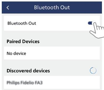
3 Devices that are paired previously will be shown in Paired devices and not paired devices will be shown in Discovered devices.
