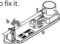
3 Install the stylus cover to protect the stylus tip.
